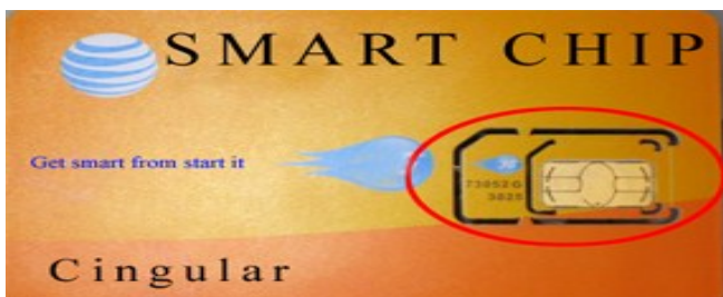
Fig. 1- Old SIM card as a credit card sized with a smaller SIM chip in it
