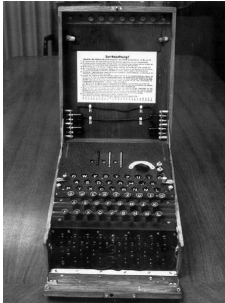
Exhibit 1-4 The German Enigma coding machine.
