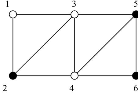
Figure 3. A 6-node network with the cut  $\{\{1, 3, 4\}, \{2, 5, 6\}\}$ .
