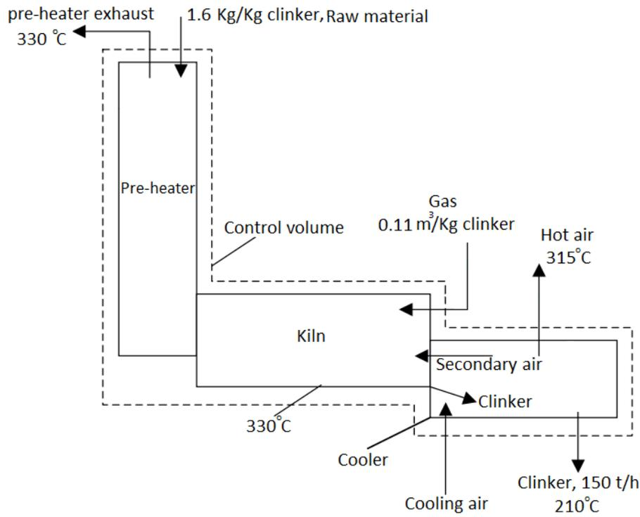
Fig. 1. Control volume, various streams and components for kiln system
