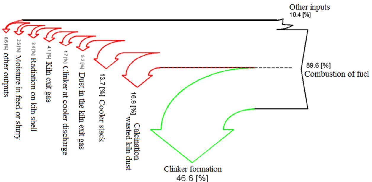
Fig. 2. The energy balance diagram (Sankey Diagram) for the layout of the curing part of the cement industry
