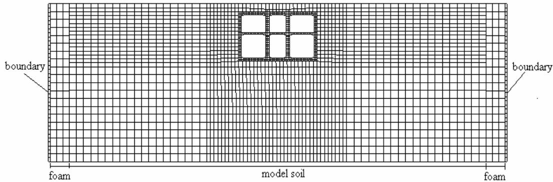
Fig.2 Meshes of soil- subway station structure system in two dimensional finite element analysis
