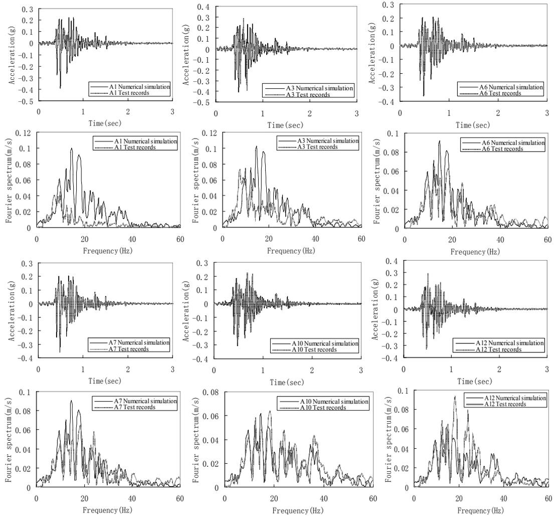
Fig.5 Acceleration time-history and Fourier spectra in different depth of model site under C-K1 test condition
