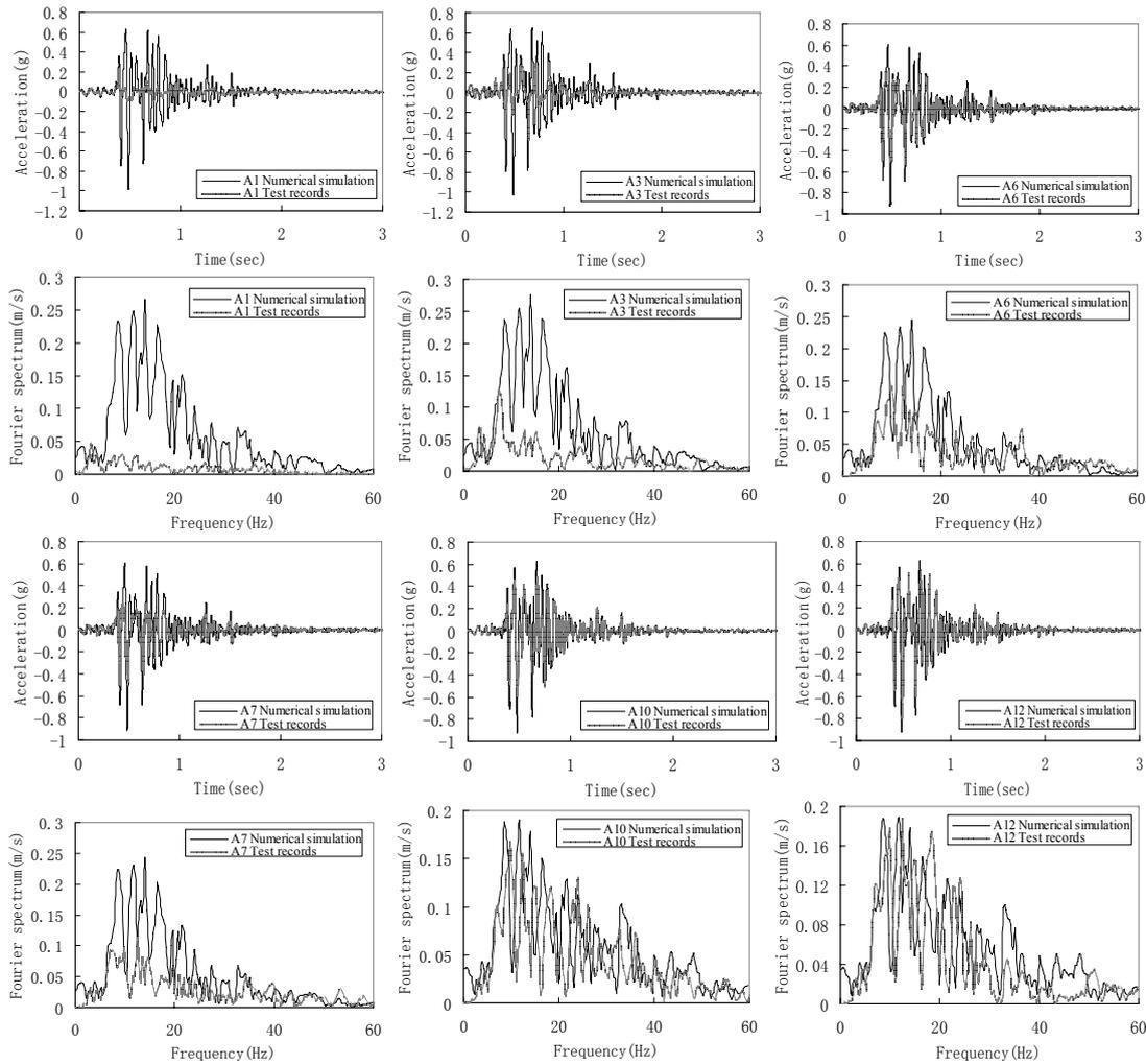
Fig.6 Acceleration time-history and Fourier spectra in different depth of model site under C-K3 test condition
