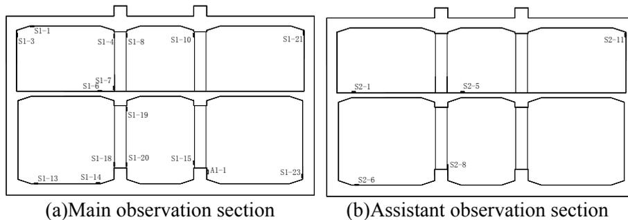
Fig.7 Distribution map of normal strain sensors in sections of subway station
