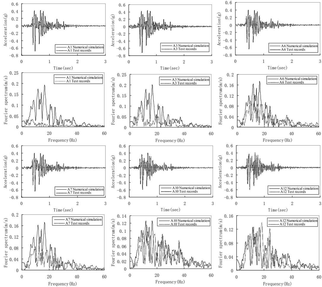
Fig.3 Acceleration time-history and Fourier spectra in different depth of model site under C-K2 test condition
