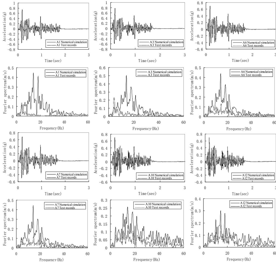
Fig.4 Acceleration time-history and Fourier spectra in different depth of model site under C-E2 test condition
