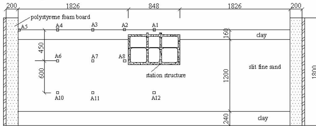
Fig.1 Schematic section of subway station structure and site model, arrangement of accelerometers (unit: mm)
