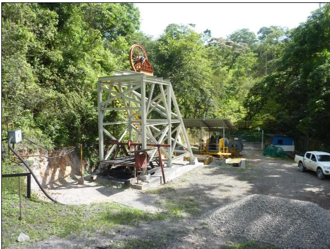
Figure 16.13 – Shaft headframe installed over 2.7 m borehole - Bonanza raise bore hole (shaft) to 1100L
