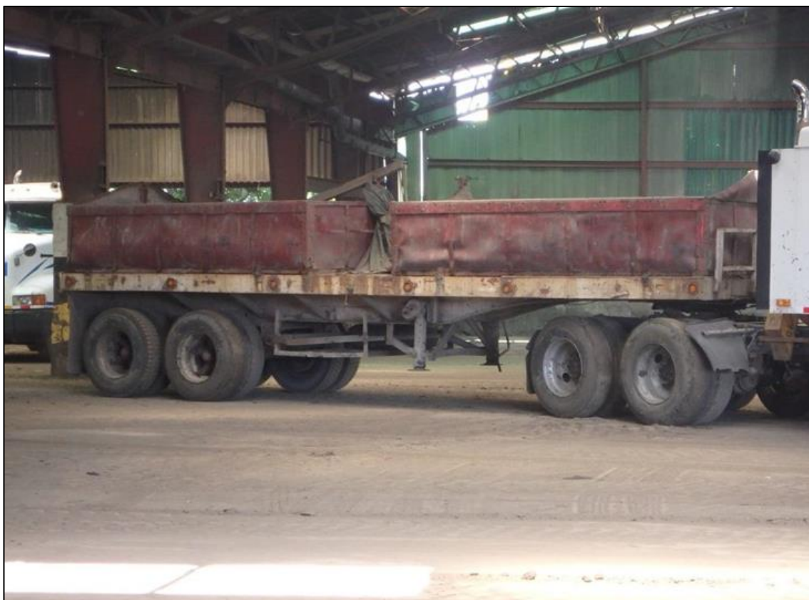
Figure 17.12 – Steel bins for concentrate transport
