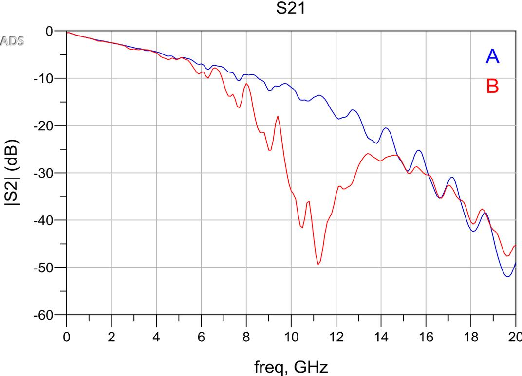
Figure 4.2 Transmission parameters for a link where the traces are routed at different levels.
