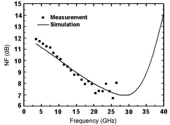
Fig. 14. Measured and simulated noise figure (NF).
