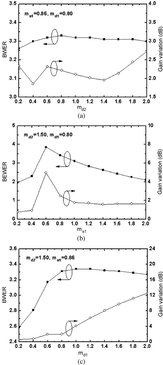
Fig. 5. The BWER and gain variation with different PIP inductors (a)  $m_{d2}$ , (b)  $m_{s1}$ , and (c)  $m_{d1}$ .
