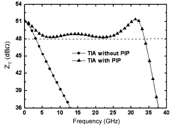
Fig. 8. Simulated frequency response for the TIA with and without PIP.
