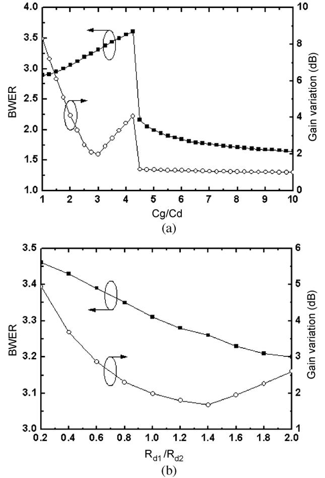
Fig. 6. The BWER and gain variation for different values of (a)  $C_g/C_d$  and (b)  $R_{d1}/R_{d2}$ .
