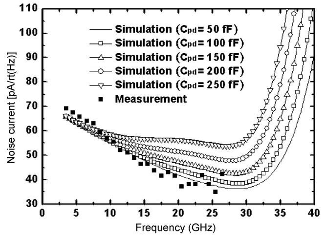
Fig. 15. Measured  $I_{n,in}$  and the simulated  $I_{n,in}$  with different values of  $C_{pd}$ .
