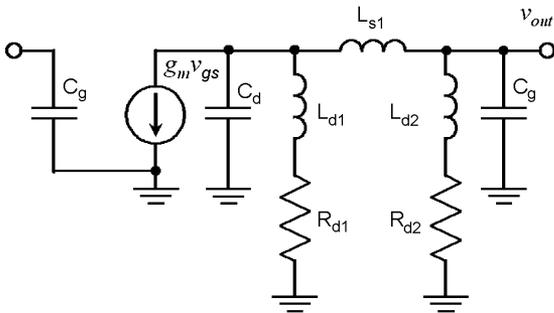
Fig. 3. The equivalent circuit model of one gain stage with the  $\pi$ -type inductor peaking (PIP) technique.
