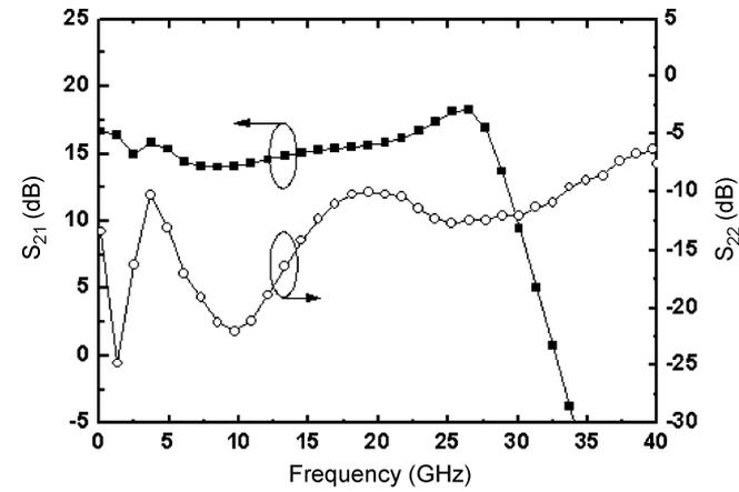
Fig. 12. Measured  $S_{21}$  and  $S_{22}$ .
