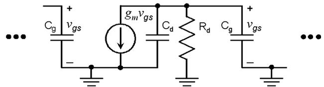
Fig. 1. Small-signal equivalent circuit model of a cascaded common-source amplifier.
