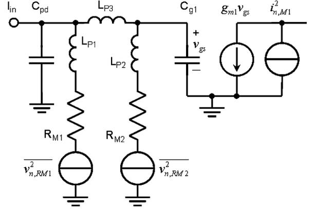
Fig. 9. Noise equivalent circuit model for the TIA input stage as shown in Fig. 7.
