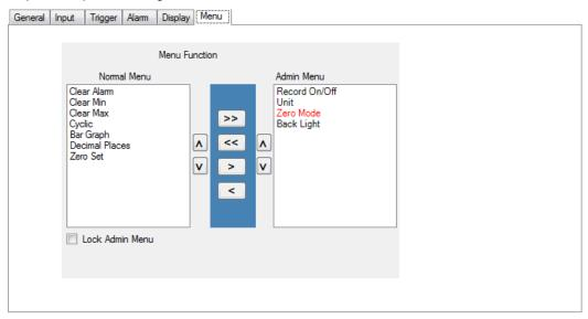
If the "Lock Admin Menu" box is checked the user will not be able to access the Admin Menu features at the Logger, and the Zero Set menu option (display offset) will not be available in the Normal Menu.
