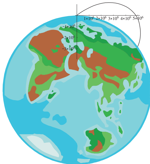
FIGURE 6.8. The projectile trajectory when there is no air drag but the velocity is fairly large.
