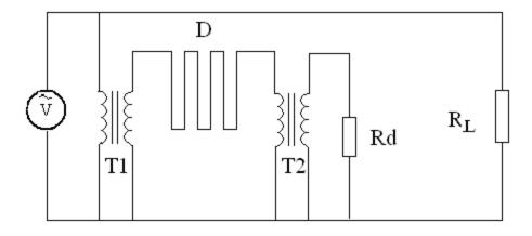
Figure 1: Schematic of combined source with single wire phase retarded circuit.
