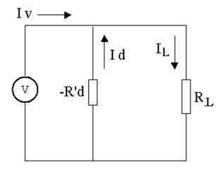
Figure 2: The equivalent circuit of the combined source and load resistor.
