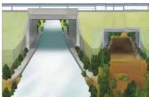
Fauna passage zones in box culvert, figure to the right shows an alternative dry passage, which does not alter the hydraulic properties of the structure.
