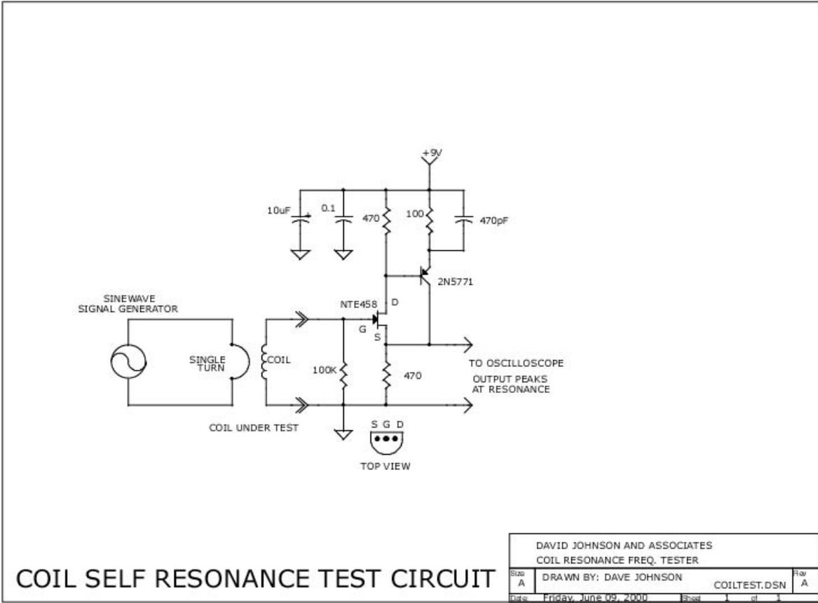
**COIL SELF RESONANCE TEST CIRCUIT**
