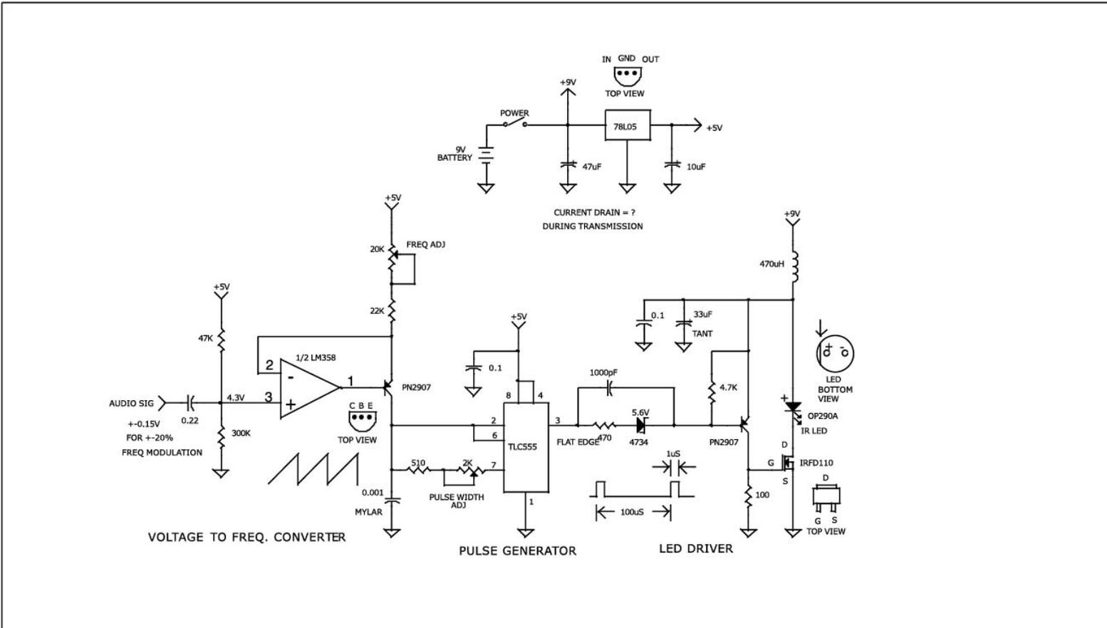
OPTICAL THROUGH THE AIR TRANSMITTER
