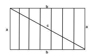
Woodworkers must make sure that the sides, tops, and bottoms of casework are square to each other during assembly. In this sense, square means that the parts are at right angles to each other.
