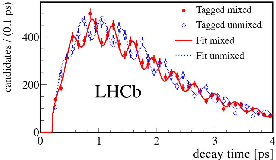
Figure 24: Decay time distribution for  $B_s^0 \rightarrow D_s^- \pi^+$  candidates tagged as mixed (different flavour at decay and production; red, continuous line) or unmixed (same flavour at decay and production; blue, dotted line) [65].
