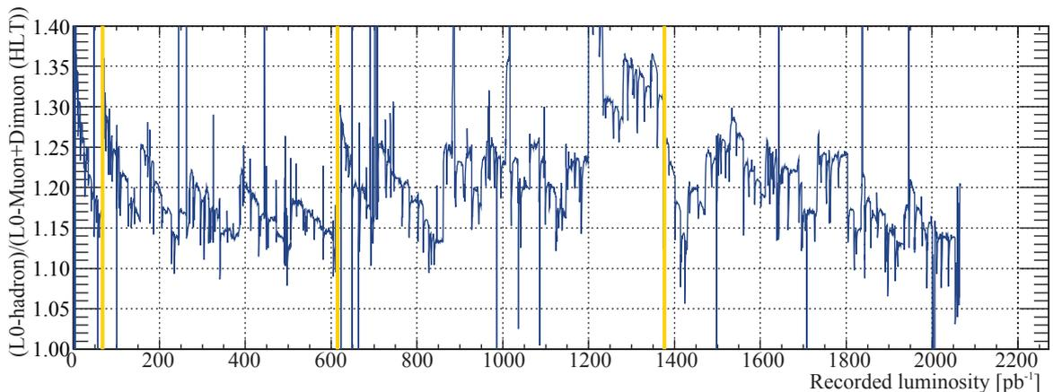
Figure 29: Ratio between the rate of events triggered by the L0-hadron trigger, based on the HCAL, and Muon-based triggers. Distinct increases in rate, *e.g.* as at a recorded luminosity of around  $50 \text{ pb}^{-1}$ , correspond to the application of a new set of PMT gains.
