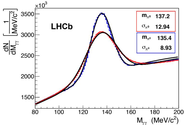
Figure 28: Invariant mass distribution for  $\pi^0 \rightarrow \gamma\gamma$  candidates upon which the fine calibration algorithm is applied. The red curve corresponds to the distribution before applying the method, while the blue curve is the final one. Values in the red (blue) box are the mean and sigma of the signal peak distribution in  $\text{MeV}/c^2$  before (after) applying the fine calibration method.
