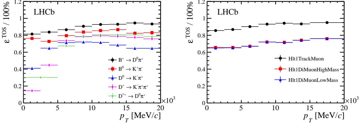
Figure 45: HLT1 inclusive track trigger performance: TOS efficiency for various channels as a function of  $B$  or  $D$   $p_T$  (left). HLT1 muon trigger performance: TOS efficiency for  $B^+ \rightarrow J/\psi K^+$  candidates as function of  $B^+$   $p_T$  (right).
