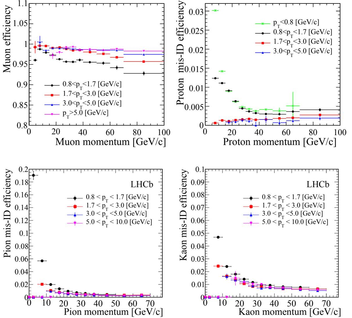
Figure 41: Top left: efficiency of the muon candidate selection based on the matching of hits in the muon system to track extrapolation, as a function of momentum for different  $p_T$  ranges. Other panels: misidentification probability of protons (top right), pions (bottom left), and kaons (bottom right) as muon candidates as a function of momentum, for different  $p_T$  ranges.
