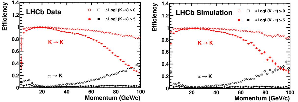
Figure 39: Kaon identification efficiency and pion misidentification rate as measured using data (left) and from simulation (right) as a function of track momentum [81]. Two different  $\Delta\log\mathcal{L}(K - \pi)$  requirements have been imposed on the samples, resulting in the open and filled marker distributions, respectively.
