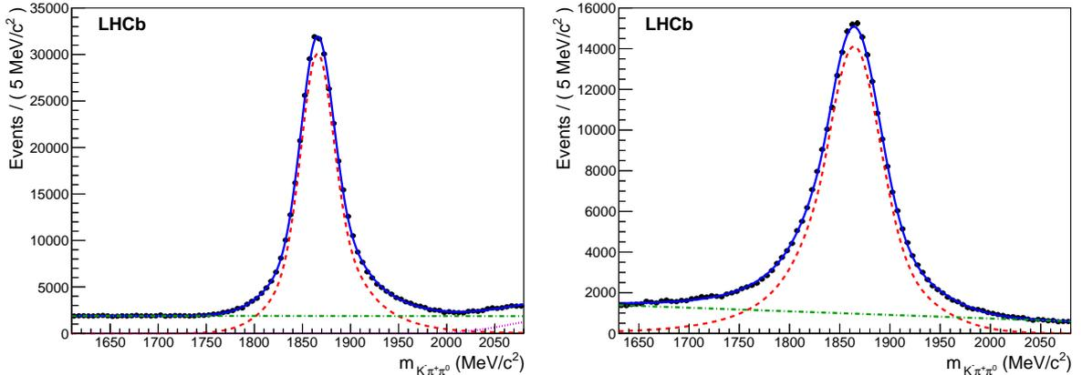
Figure 31: Mass distributions of reconstructed  $D^0 \rightarrow K^- \pi^+ \pi^0$  candidates with resolved  $\pi^0$  (left) and merged  $\pi^0$  (right). Both are obtained from the 2011 data sample. The overall mass fit [78] is represented by the blue curve, with the signal (red dashed line) and background (green dash-dotted line and purple dotted lines) contributions also shown.
