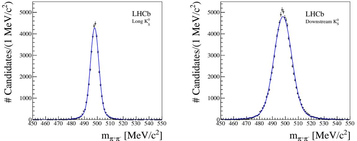
Figure 27: Distribution of the invariant mass of  $K_S^0 \rightarrow \pi^+\pi^-$  candidates with a decay vertex at a significant distance to the PV, for long tracks (left) and downstream tracks (right). A mass resolution of  $3.5 \text{ MeV}/c^2$  is achieved for the candidates reconstructed from long tracks and  $7 \text{ MeV}/c^2$  for those using downstream tracks.
