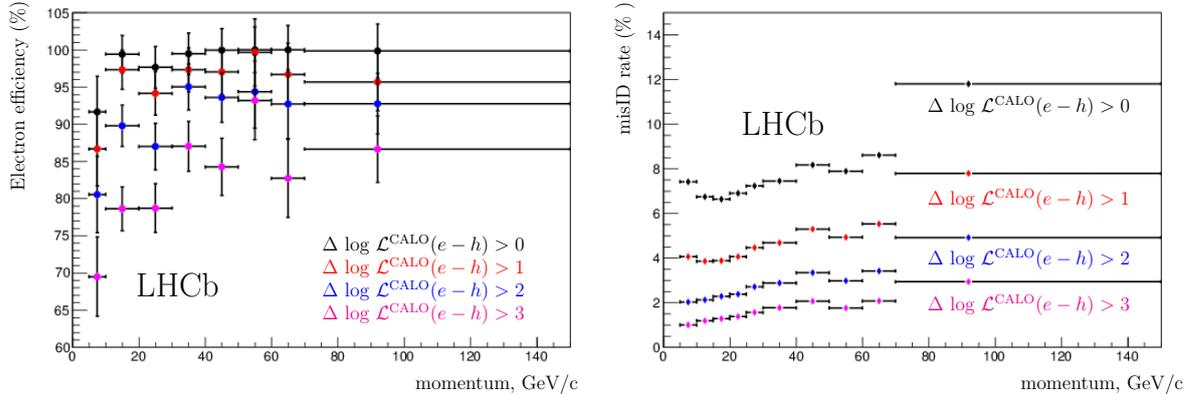
Figure 36: Electron identification performances for various  $\Delta \log \mathcal{L}^{\text{CALO}}(e-h)$  cuts: electron efficiency (left) and misidentification rate (right) as functions of the track momentum.
