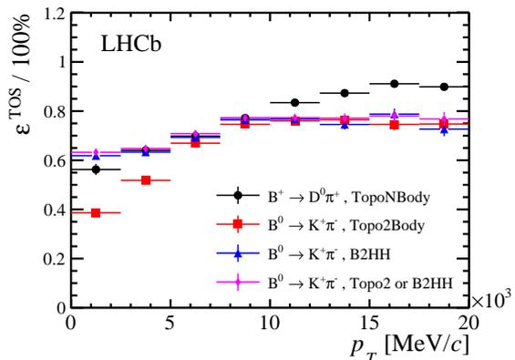
Figure 47: HLT2 inclusive beauty trigger performance as a function of  $B p_T$ . The efficiency for the exclusive  $B^0 \rightarrow K^+ \pi^-$  trigger line is also given.
