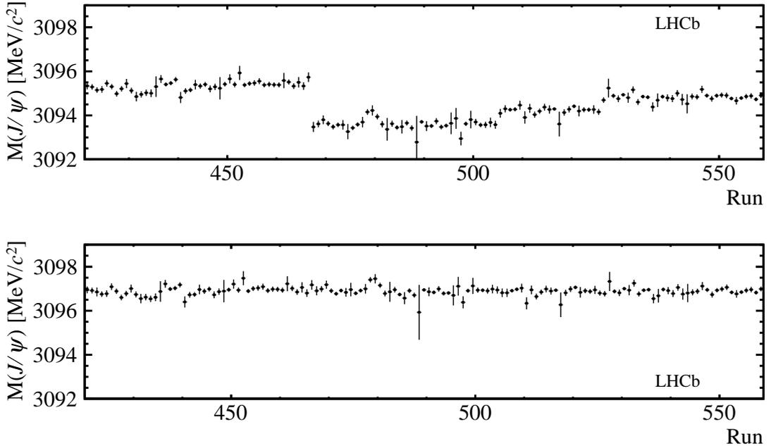
Figure 22: Fitted position of the peak of the  $J/\psi \rightarrow \mu^+\mu^-$  invariant mass distribution as a function of run number in a two-week period in which the operating temperature of TT modules was varied. The mass is evaluated using the same alignment for the full period on the top and using a dedicated track alignment for each period with constant temperature on the bottom.
