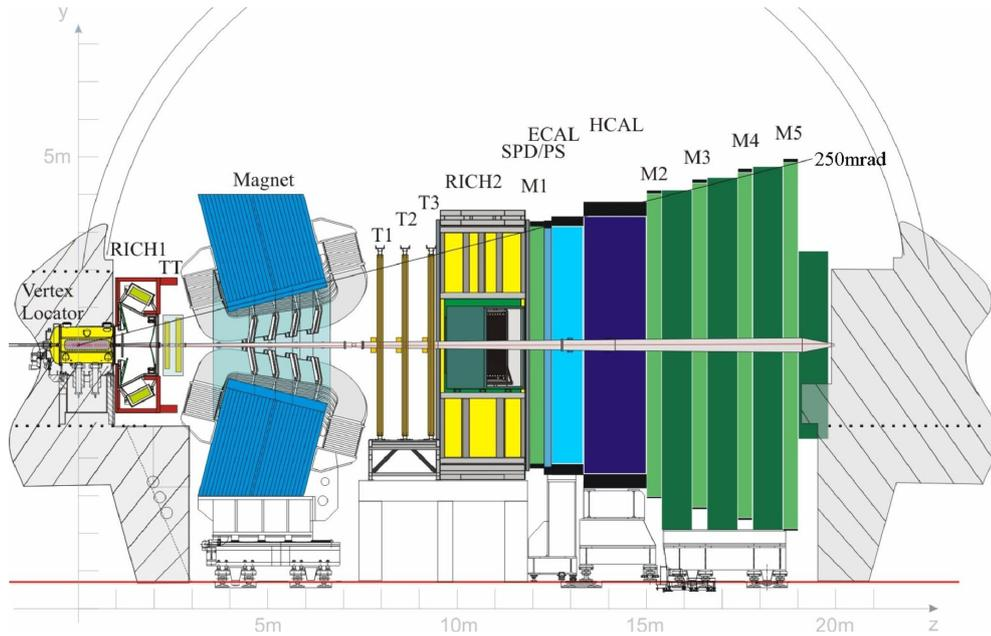
Figure 1: View of the LHCb detector [23].
