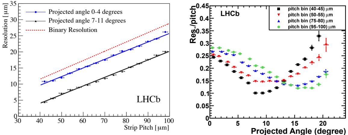
Figure 5: The VELO hit resolution as a function of the inter-strip pitch (left) evaluated with 2010 data for the  $R$  sensors. Results are shown for two projected angle ranges and the expected resolution of a single-hit binary system is indicated for comparison. Resolution divided by pitch as a function of the track projected angle for four different strip pitches (right).
