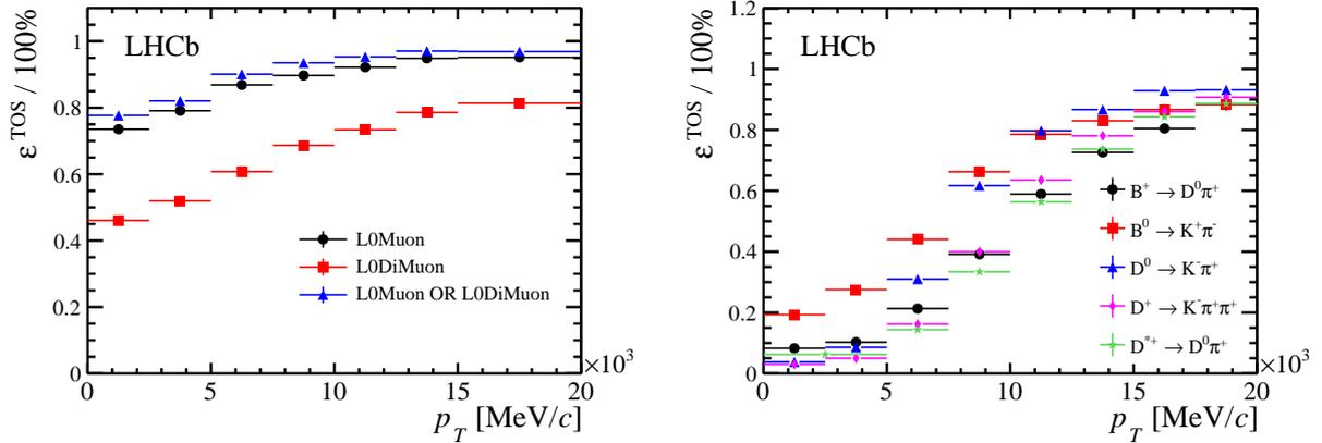
Figure 44: (left) L0 muon trigger performance: TOS trigger efficiency for selected  $B^+ \rightarrow J/\psi K^+$  candidates. (right) L0 hadron trigger performance: TOS trigger efficiency for different beauty and charm decay modes.
