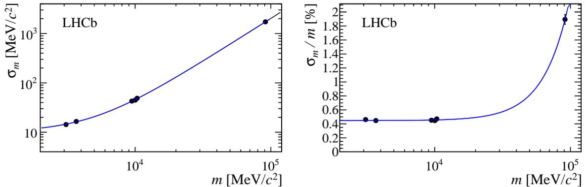
Figure 19: Mass resolution ( $\sigma_m$ ) (left) and relative mass resolution (right) as a function of the mass ( $m$ ) of the dimuon resonance. The mass of the muons can be neglected in the invariant mass calculation of these resonances. The mass resolution is obtained from a fit to the mass distributions. The superimposed curve is obtained from an empirical power-law fit through the data points.
