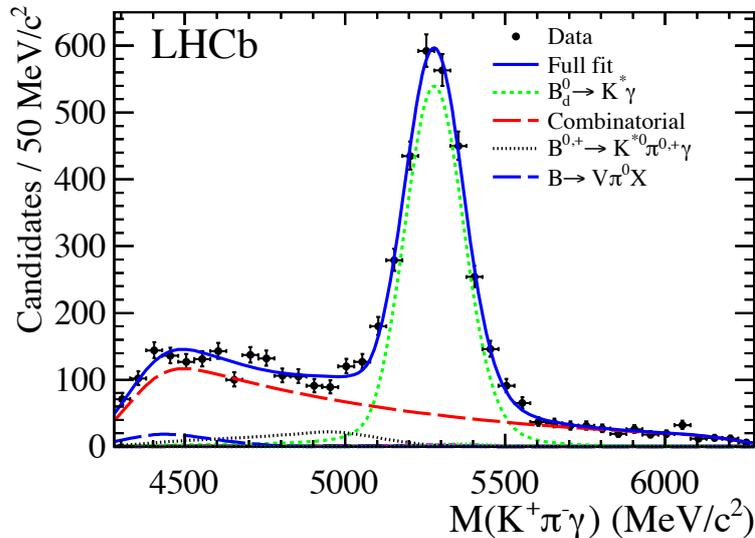
Figure 30: Mass distribution of reconstructed  $B^0 \rightarrow K^{*0}(K^+\pi^-)\gamma$  candidates obtained in the 2011 data sample. The blue curve corresponds to the mass shape fit. The  $K^{*0}\gamma$  signal (green dotted line) and the various background contaminations are shown [77].
