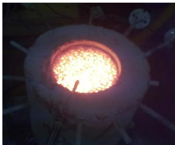
Fig. 3. A submerged flame inside SiC foam
