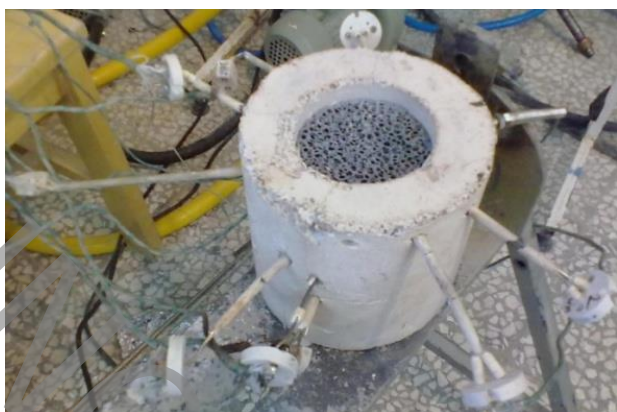
Fig. 2. The position of the thermocouples on the retainer
