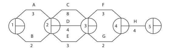
(a) Using the data in the network diagram above, calculate the Earliest Start Times (EST) and Latest Finishing Times (LFT) for each activity and identify the critical path.
