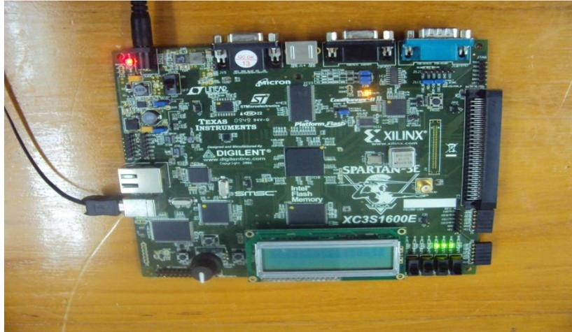
Fig. 5. Spartan-3E FPGA development kit
