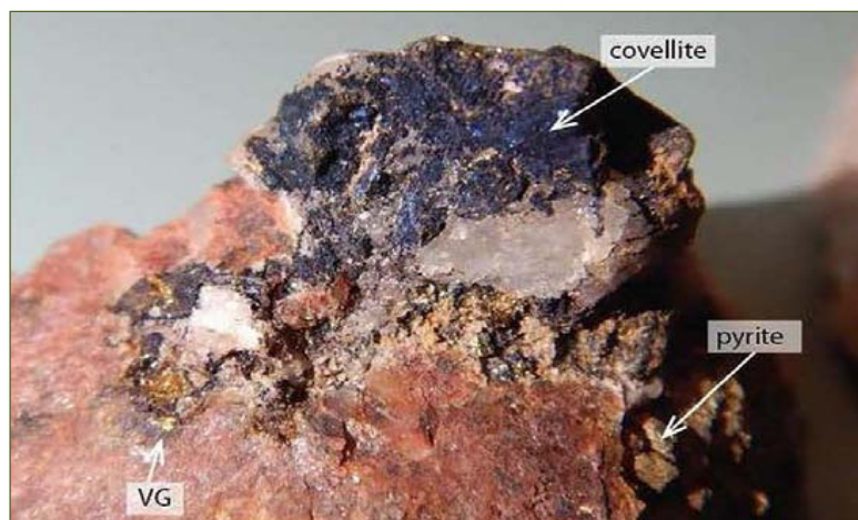
High-grade quartz-pyrite-covellite-gold vein
