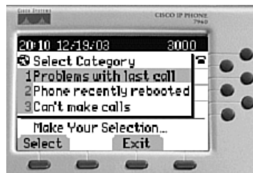
Figure 7-7 QRT Menu Choices When the Phone Is On-Hook
