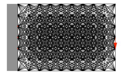
Each link represents a rigid rod that has a thickness, with its weight proportional to the force on it and its length. The aim is to minimize the total material used, which is
