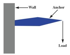
This problem can be modeled by discretizing and simulating it using nodes and links. The modeling process is illustrated using the following figure. Here a grid of  $7 \times 10$  nodes is generated. Each node is then connected by a link to all other nodes that are of Manhattan distance of less than or equal to three. The three red nodes are assumed to be fixed to the wall, while on all other nodes, compression and tension forces must balance.
