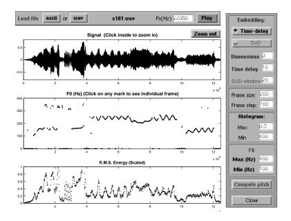
Figure 8: Terez's algorithm with subharmonic errors (singing).
