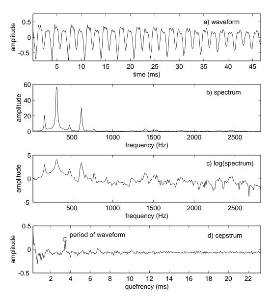
Figure 6: Stages in the cepstrum analysis algorithm.
