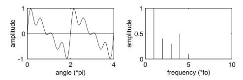
Figure 2: Waveform with lower power upper harmonics.
