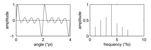
Figure 3: Waveform with higher power upper harmonics.
