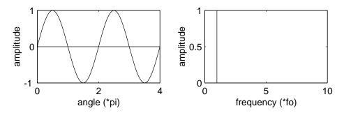
Figure 1: Waveform with no upper harmonics.
