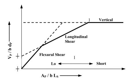
Figure 2 (b). Three modes of failure of composite slab
