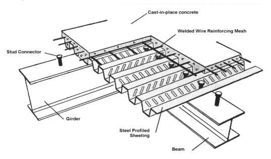
Figure 1. Details of composite profiled deck slab
