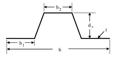
Figure 3. Cross section of trapezoidal profile (pitch length)
