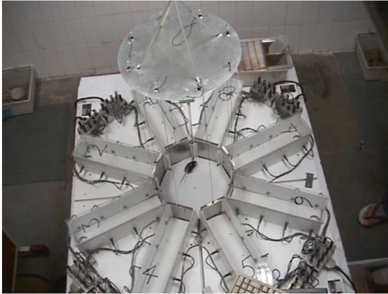
Fig. 146.3 Radial arm maze. A photograph of Radial Arm Maze apparatus at the National Brain Research Centre. Radial Arm Maze is an apparatus first designed by Samuel and Olton (1976). The apparatus is used to study spatial memory in laboratory animals or human subjects. The picture shows radial arm maze used for studying spatial memory in mice. It consists of a central platform with eight arms radiating from it. At the end of each arm is food cup in which a reward (in this case a chocoflake or a small food pellet) is kept. Each arm is separated from the central platform by a Guillotine door. All the Guillotine doors are attached to common pulley. Both central platform and arms are covered with transparent plexiglass covers. Different temporal domains of spatial memory viz. reference memory, working memory can be tested by employing different experimental paradigms (Courtesy: Professor V. Ravindranath, former Director, National Brain Research Centre)
