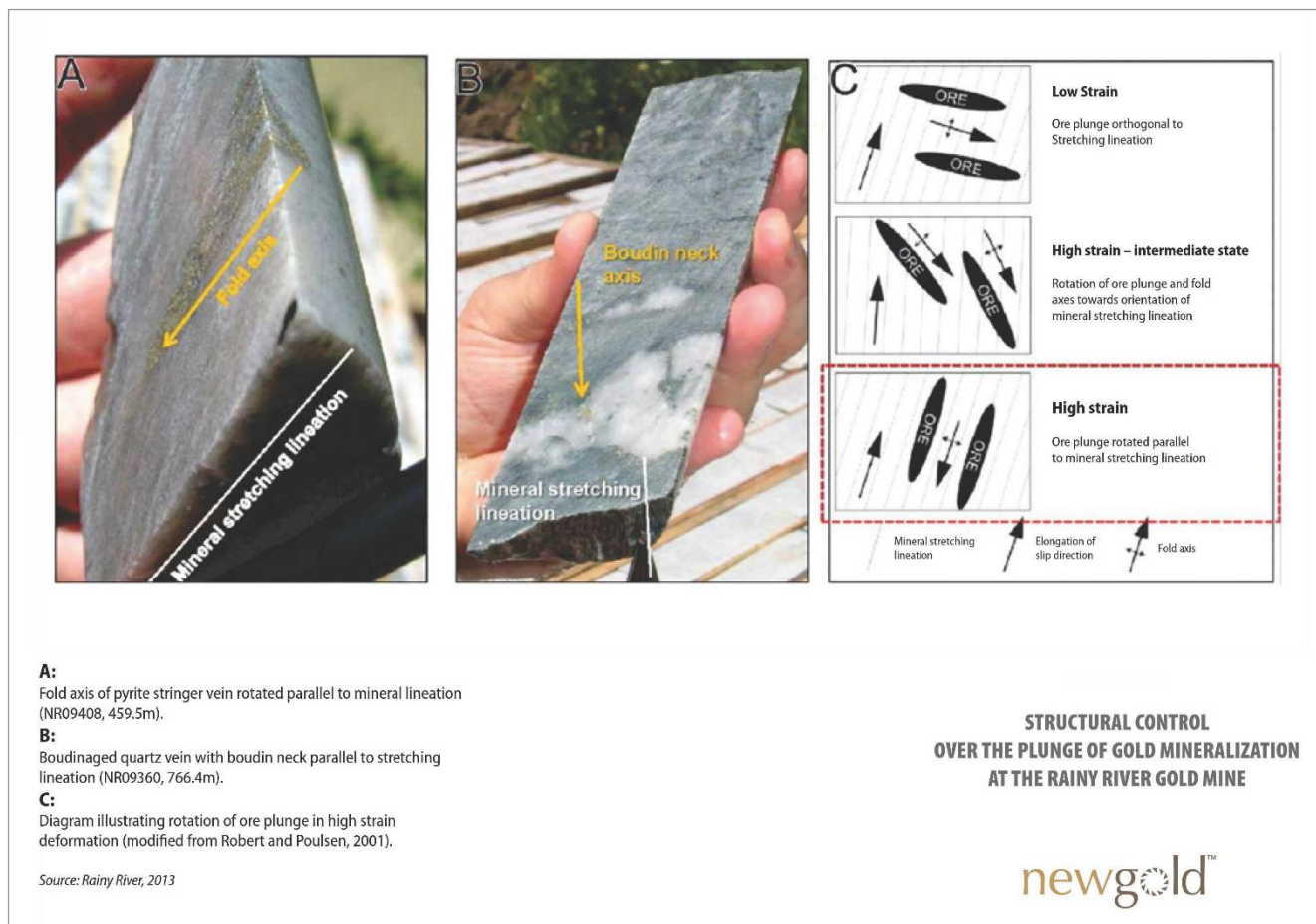
Figure 7.6 Structural control over the plunge of gold mineralization at Rainy River
