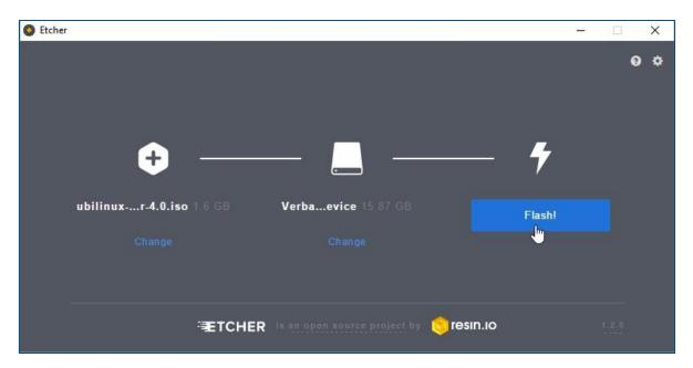
After burning the image to the USB flash drive, connect it to the UP board. Your monitor, keyboard and mouse should be already connected.
