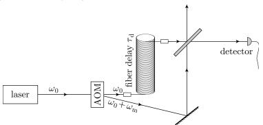
The fiber is assumed to cause a well-defined time delay of the undiffracted beam, of around 5  $\mu$ s for a 1 km fiber. (A fiber delay of the first-order beam just amounts to taking a negative  $\tau_{\rm d}$ .) For delays achievable in
