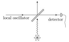
Even though this setup detects some "irrelevant" light due to the local oscillator, the amount of information that we acquire via this setup (within the idealizations below) is equivalent to that of direct detection. If the
