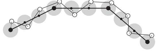
Figure 11: Basic idea of wrinkle meshes. The high resolution wrinkle mesh (white vertices) follows the low-resolution dynamic mesh (black vertices) by restricting the white vertices to remain within a certain distance (gray discs) to the dynamic mesh.
