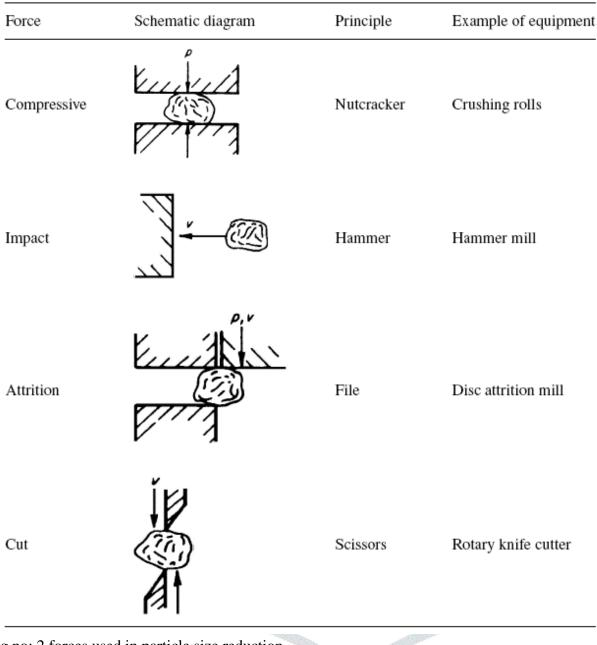
Fig no: 2 forces used in particle size reduction
