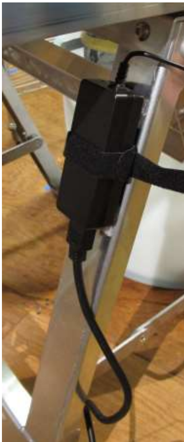
Figure 2. Power supply included with the Emriver Em2 model, shown attached to the downstream support.
