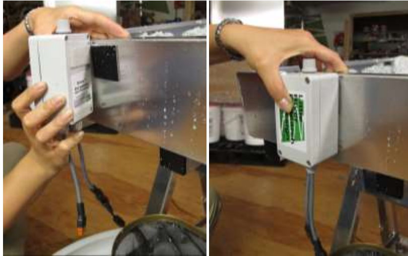
Figure 19. Attach the controller to the downstream end of the box.
