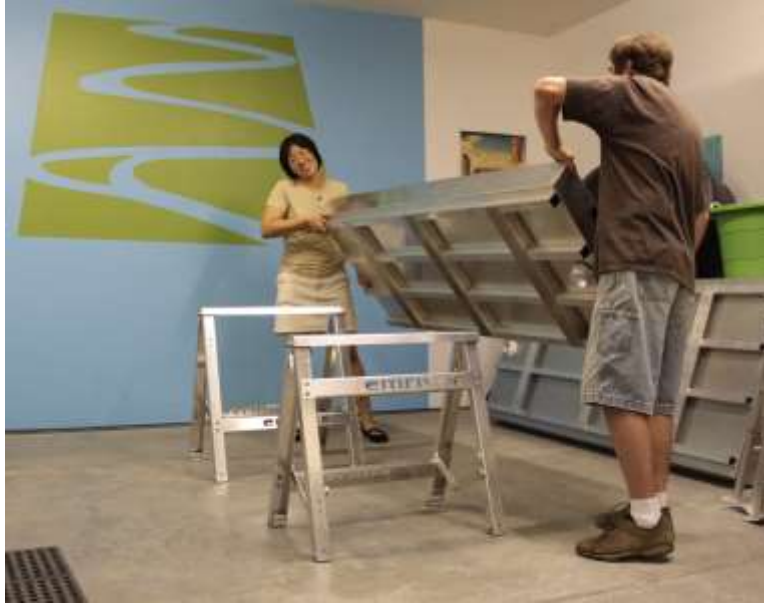
Figure 7. Lift the box onto the supports. It is best to complete this task with two people.
