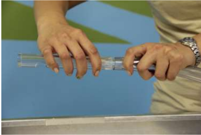
Figure 12. Insert the flow outlet into the tubing.
