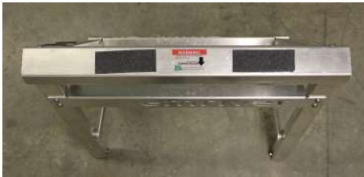
Figure 4. Labels on the supports indicate proper orientation, with the shorter support at the downstream end.
