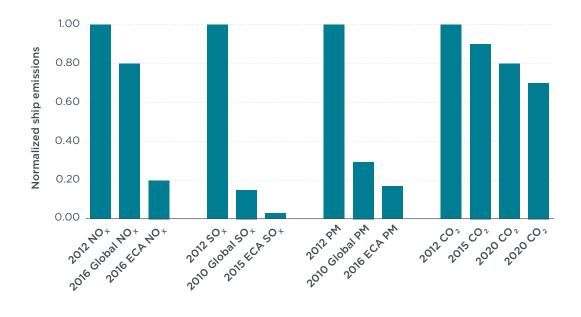
**Figure 2:** Required NO<sub>x</sub>, SOx, PM, and CO<sub>2</sub> emission reductions to meet new shipping vessel engine and fuel requirements in the 2015–25 time frame
