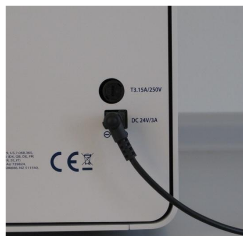
Figure 8 DC Power Plug
