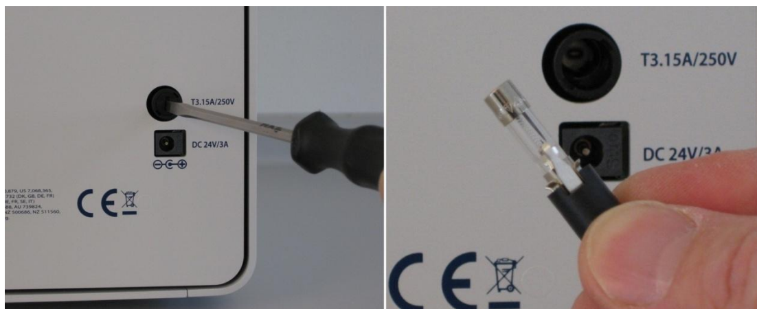
Figure 16. Location, removal and inspection of the fuse
