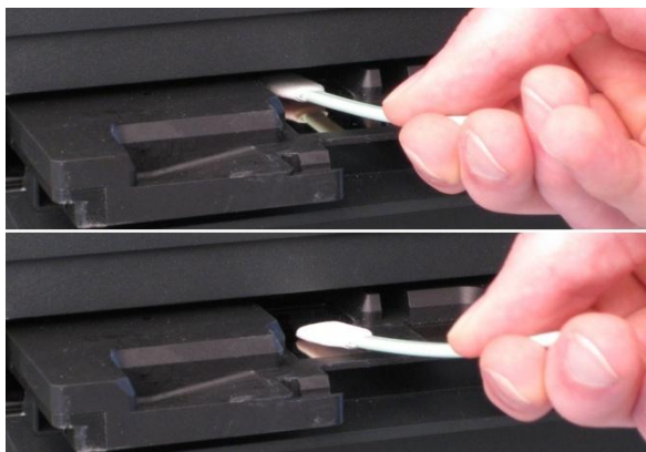
Figure 14 Illustration of how to clean the optical windows with a clean and dry Alpha Swab.
