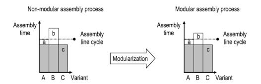
Figure 4 -The tables illustrate improved work balance achieved at the assembly station through introducing modularization. (Fredriksson, 2006)
