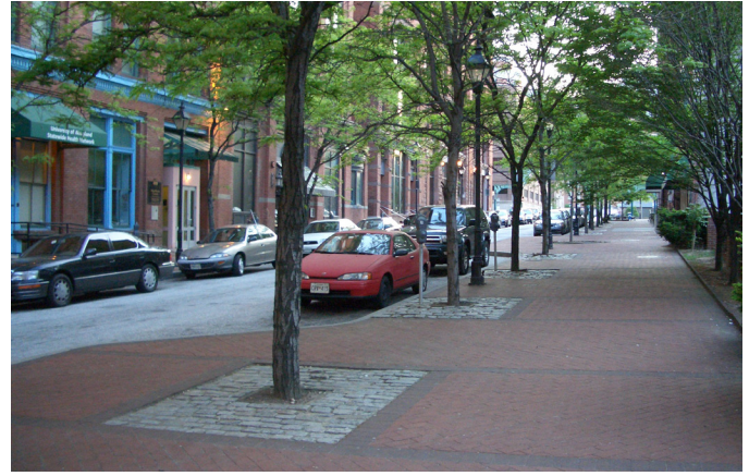
Individual pavers allow percolation of stormwater into the ground.
