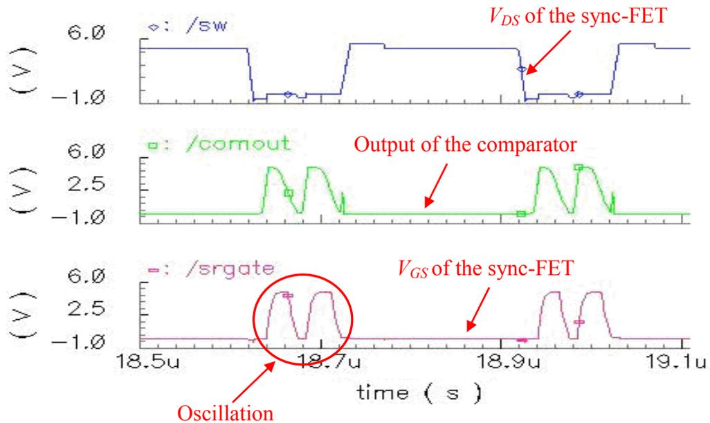
Figure 2.16 Simulation results for  $V_{OS} < 0$  without the ONE-SHOT control
