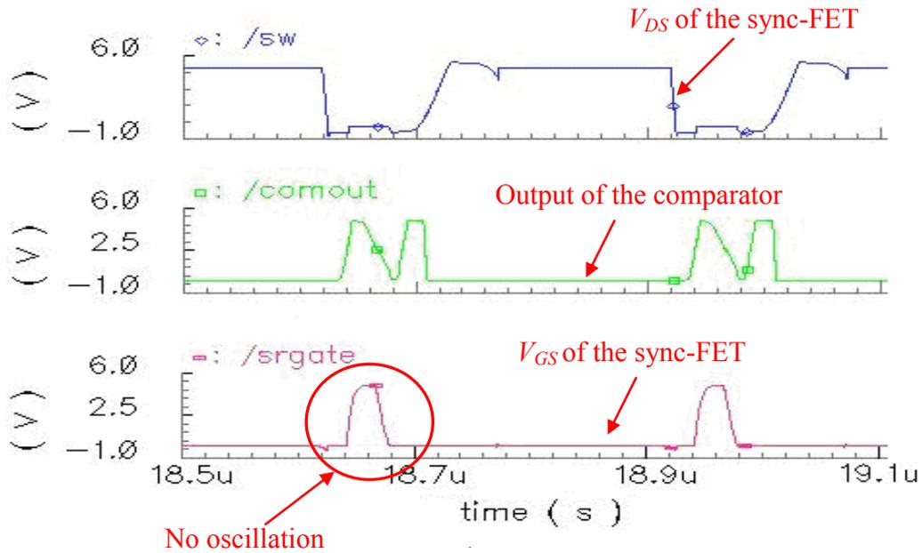
Figure 2.17 Simulation results for  $V_{OS} < 0$  with the ONE-SHOT control
