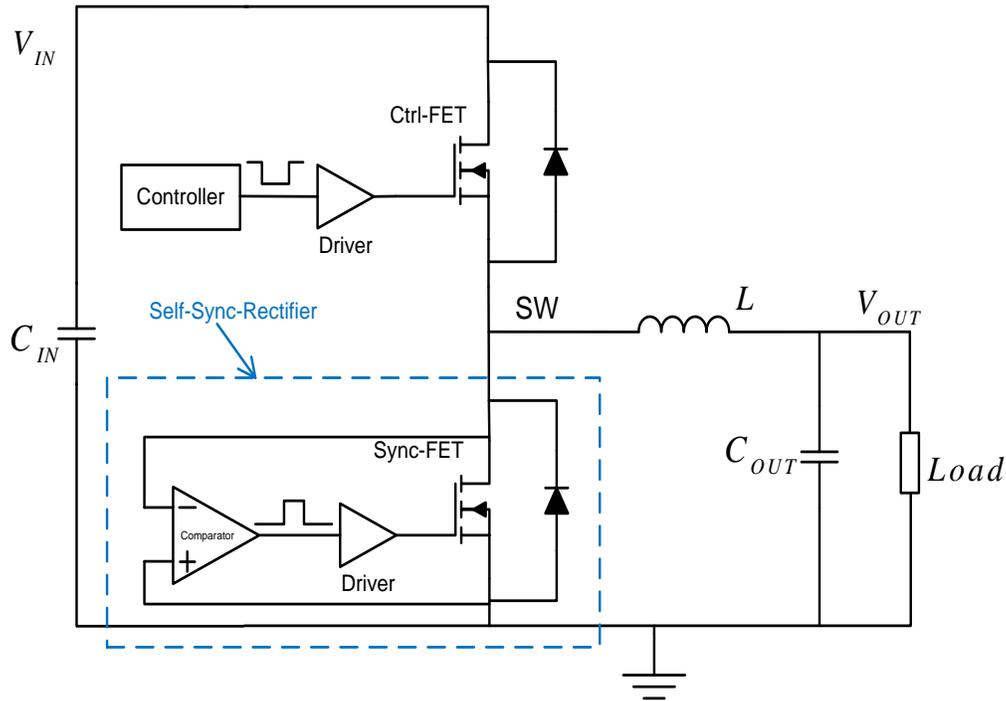
Figure 2.2 Concept of the proposed self-synchronous rectifier
