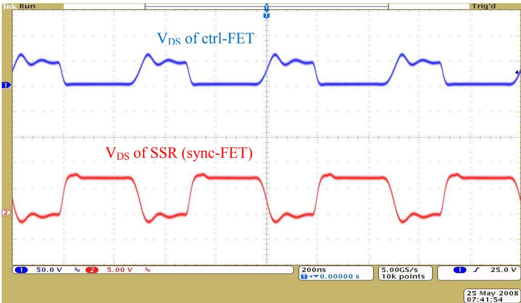
Figure 3.7 Operating waveforms at 2MHz
