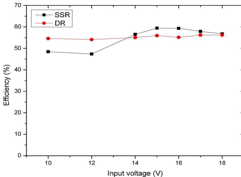
Figure 3.9 Measured efficiency vs. input voltage
