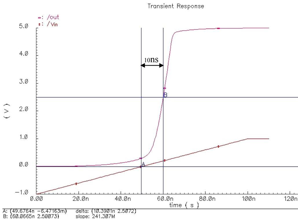
Figure 2.13 Propagation delay simulation for the voltage comparator (typ.)
