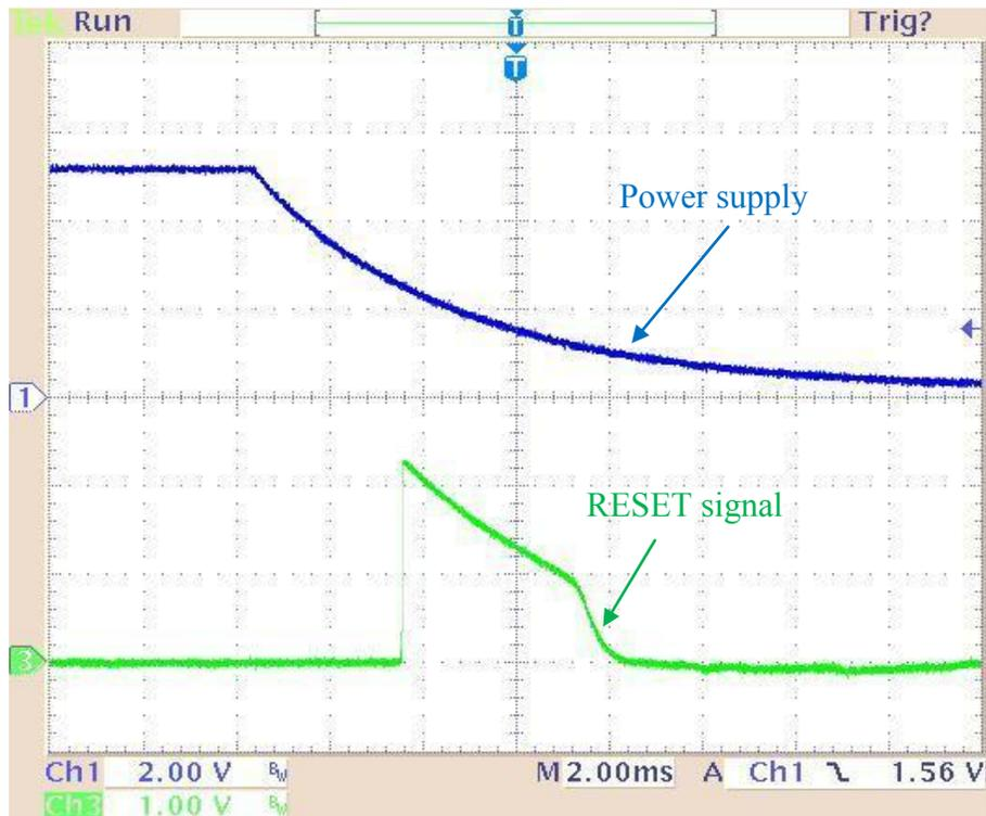
Figure 2.22 UVLO at Power-down transient
