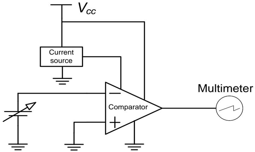
Figure 2.24 Comparator offset voltage testing setup
