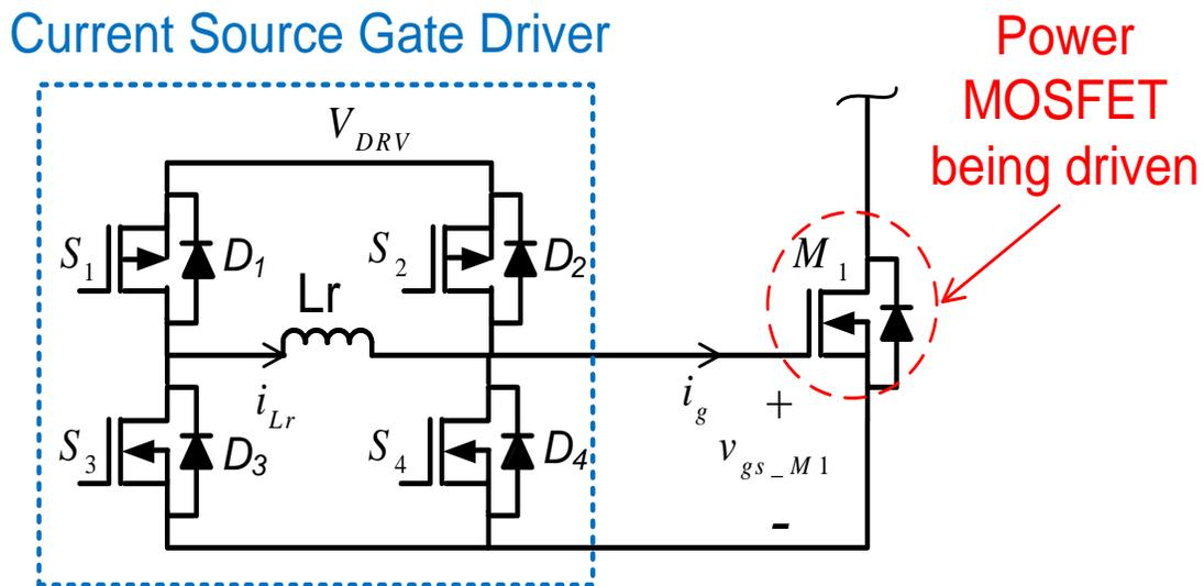
Figure 4.1 Schematic diagram of the current source driver (CSD)
