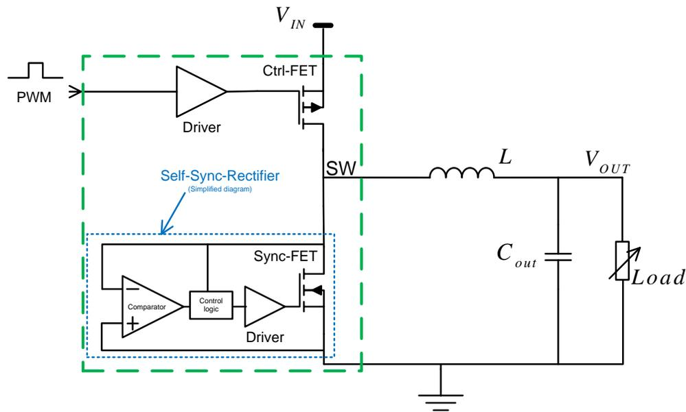
Figure 2.26 Simple buck converter testing circuit
