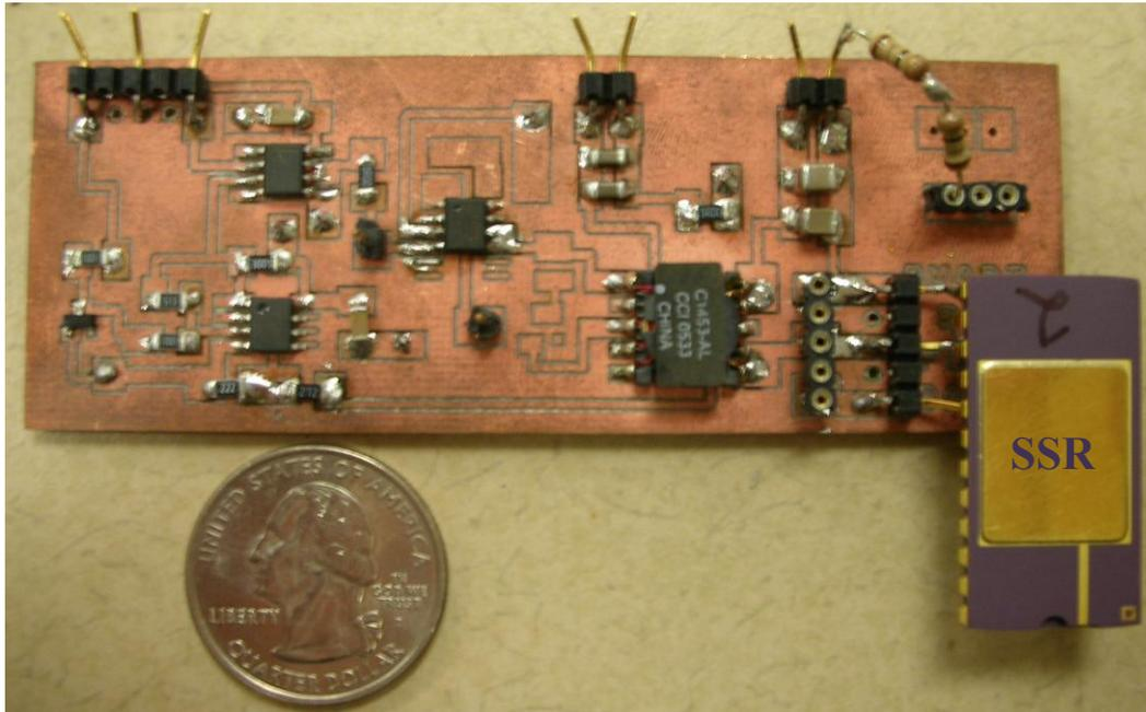
Figure 3.5 Prototype of the proposed flyback converter with the SSR
