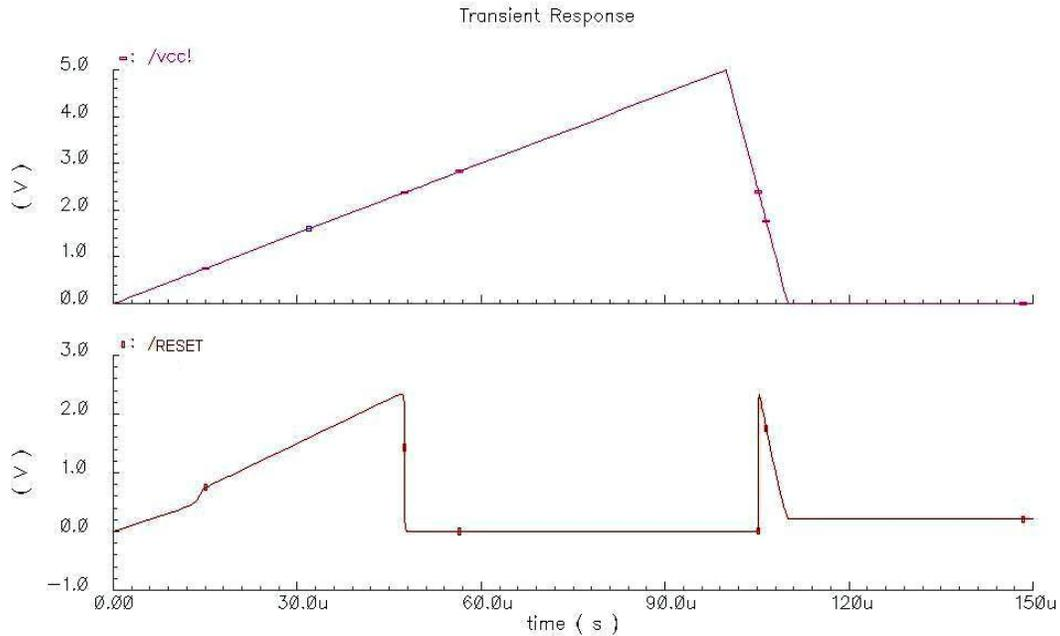
Figure 2.5 Simulated transient response of the POR (typical)
