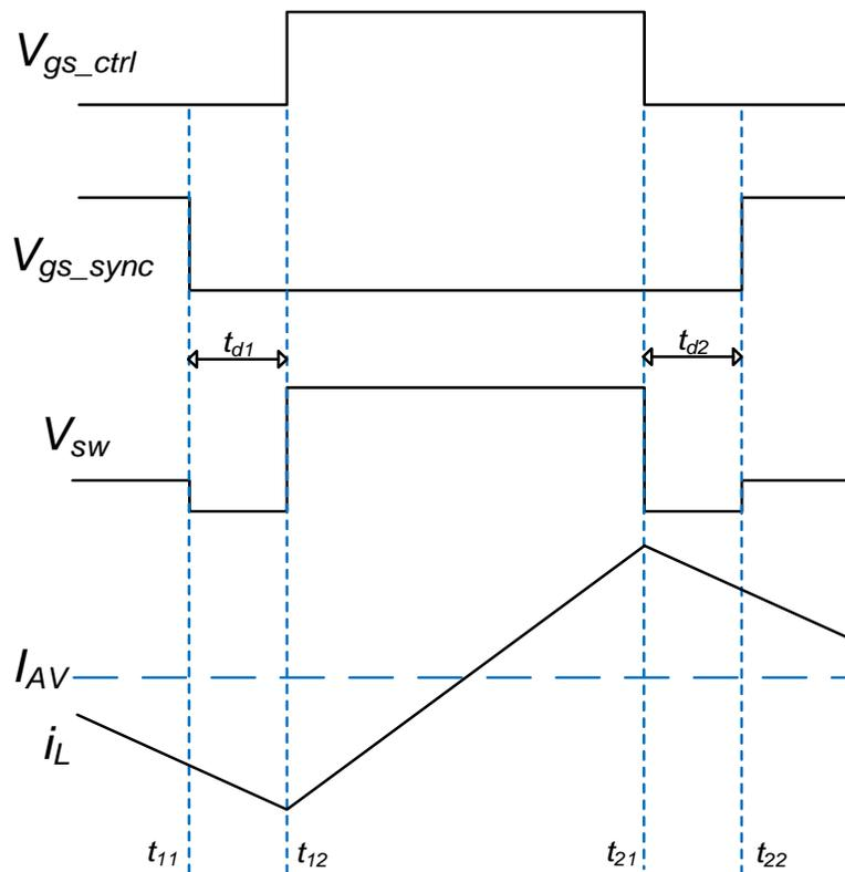
Figure 1.3 Switching waveforms of a typical synchronous buck converter
