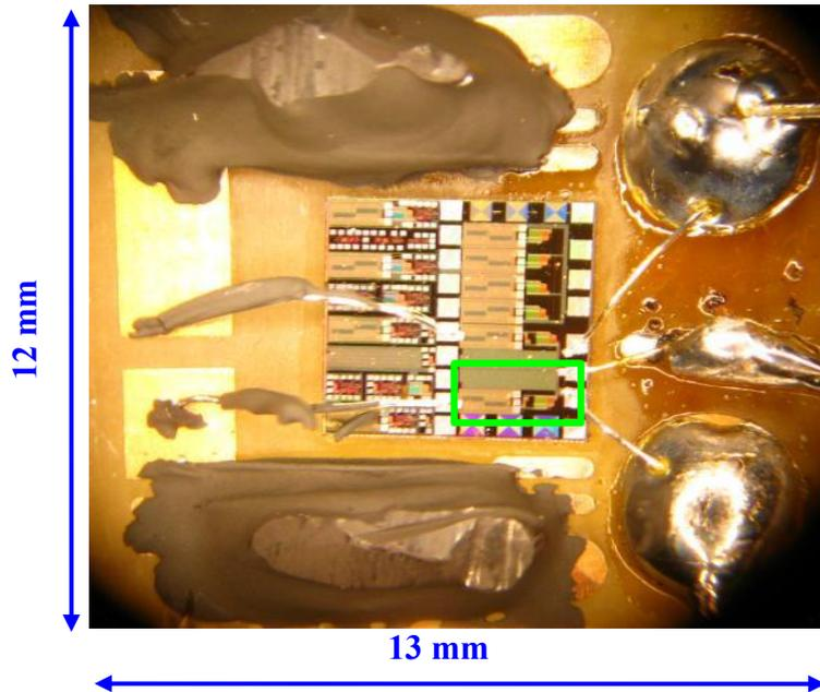
Figure 5.6 The buck PSiP after ferrite epoxy coating
