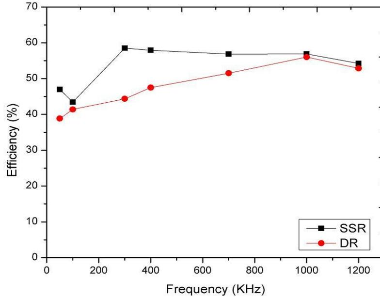
Figure 3.10 Measured efficiency vs. switching frequency
