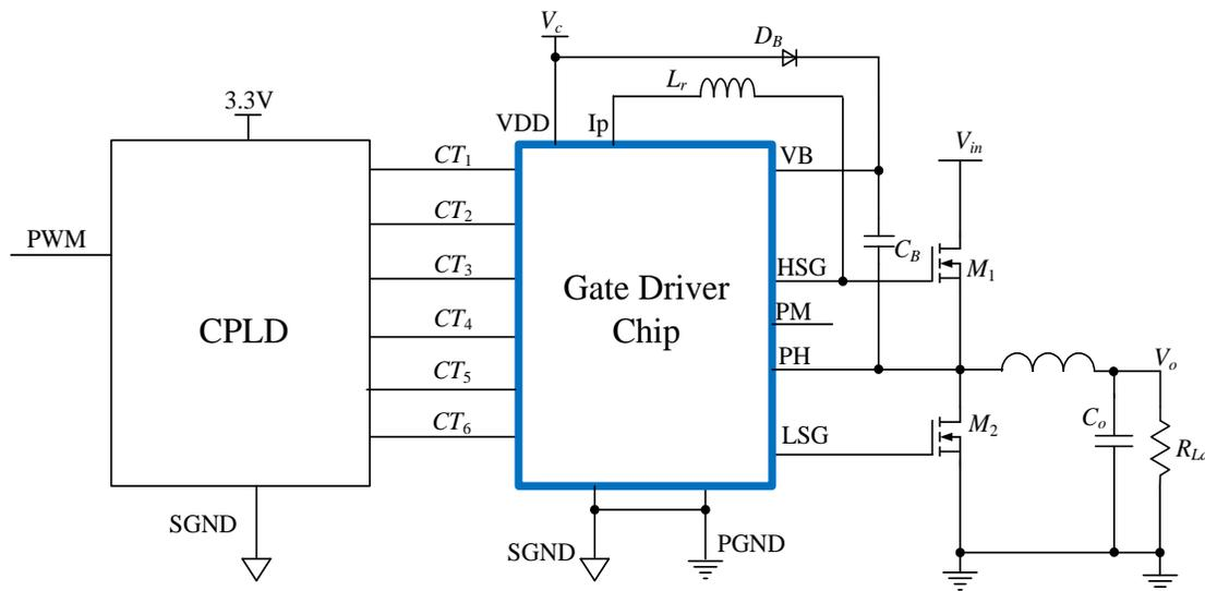
Figure 4.3 System level block diagram of a buck converter driver chip are connected to the gates of high-side MOSFET  $M_1$  and low-side MOSFET  $M_2$  in the power stage of the buck converter.
