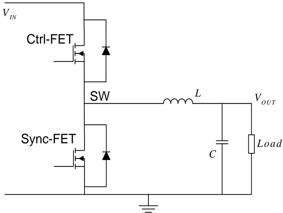
Figure 1.2 A typical synchronous buck converter
