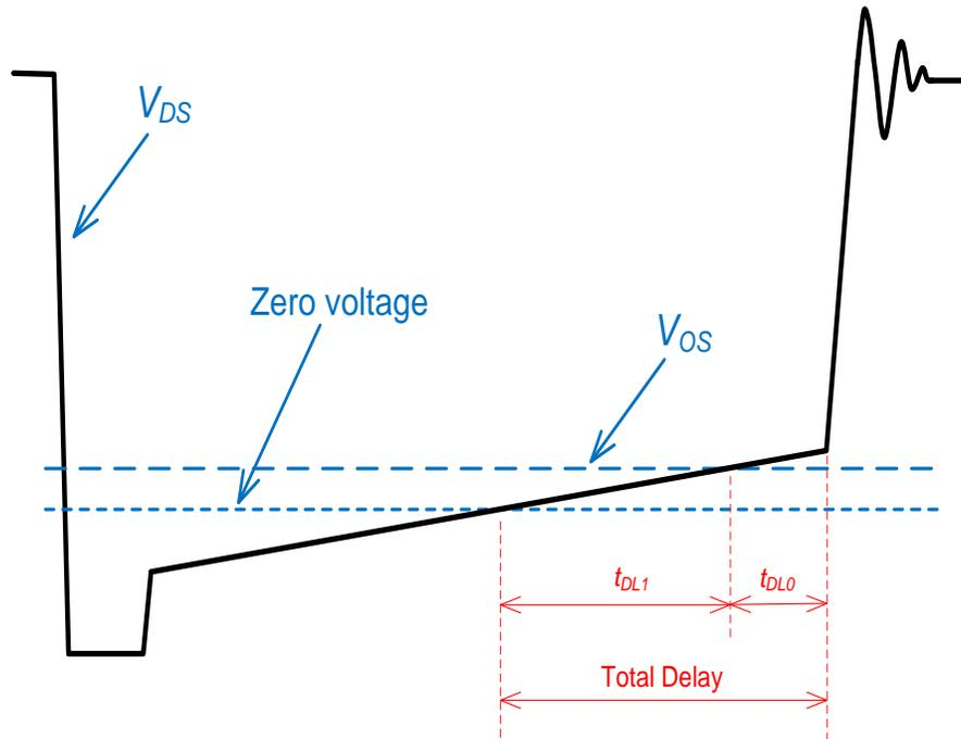
Figure 2.9  $V_{DS}$  waveform of the sync-FET for  $V_{OS} > 0$
