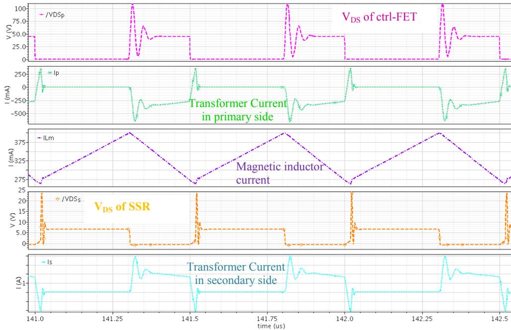
Figure 3.3 CCM Simulation
