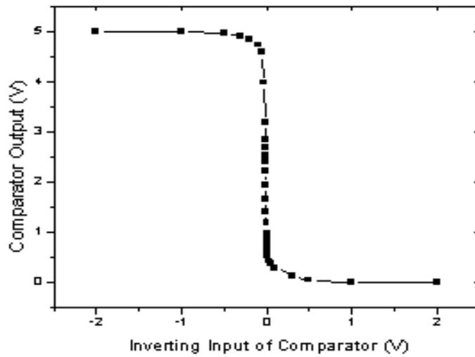
Figure 2.25 Comparator DC transfer characteristics
