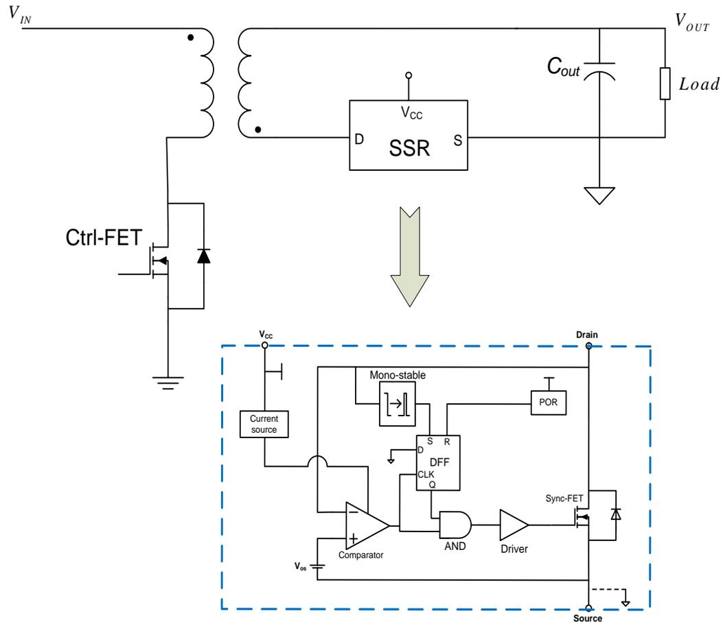
Figure 3.1 Proposed synchronous flyback converter with the SSR
