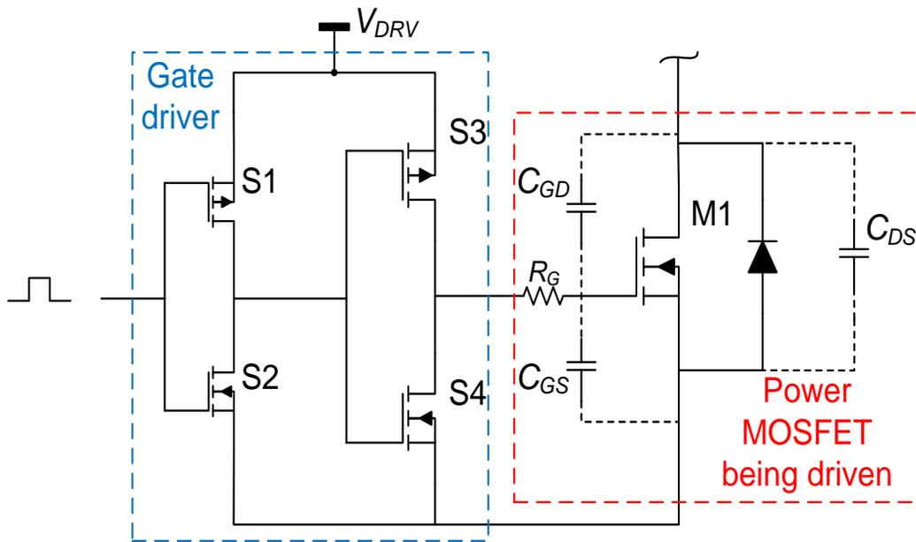
Figure 1.6 Simplified conventional gate driver
