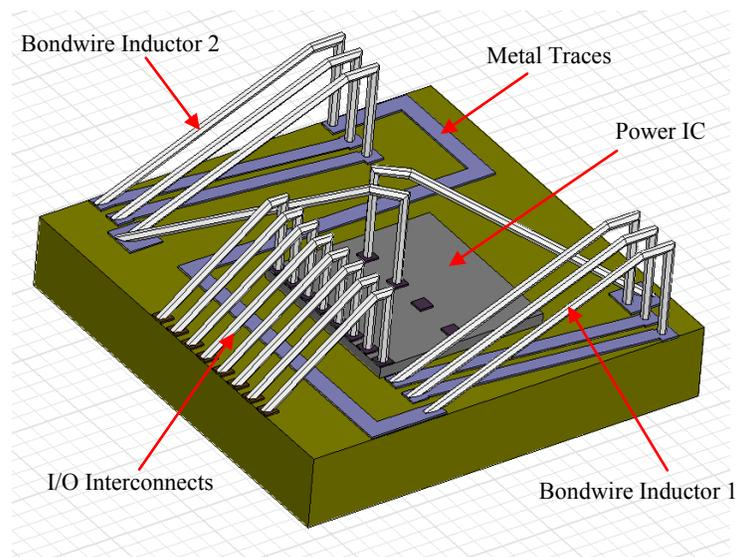
Figure 5.3 Conceptual drawing of the PSiP buck converter
