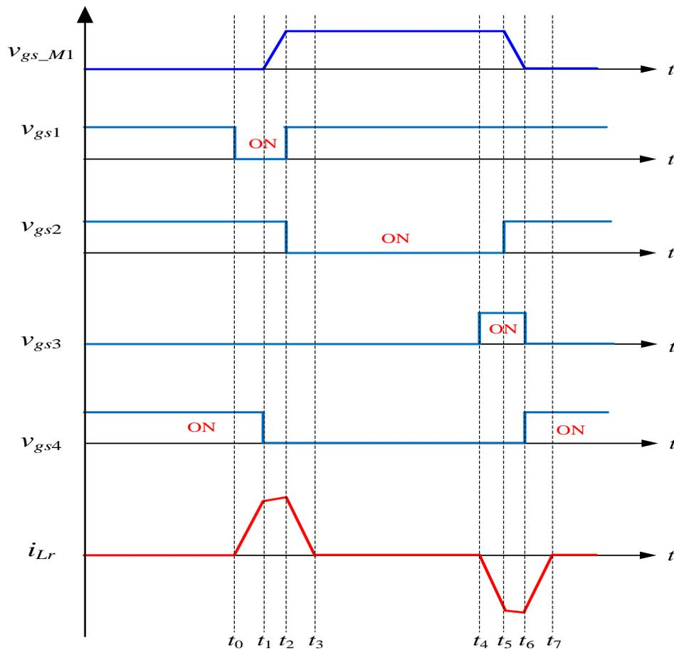
Figure 4.2 Waveforms of the CSD circuit
