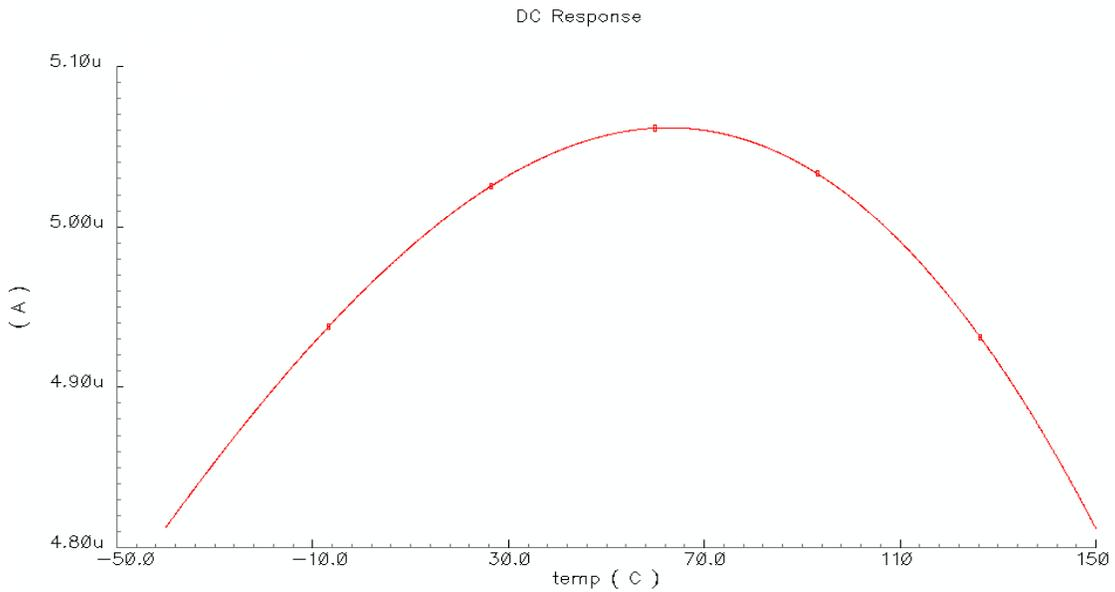
Figure 2.8 Current source temperature dependence (typ.1)
