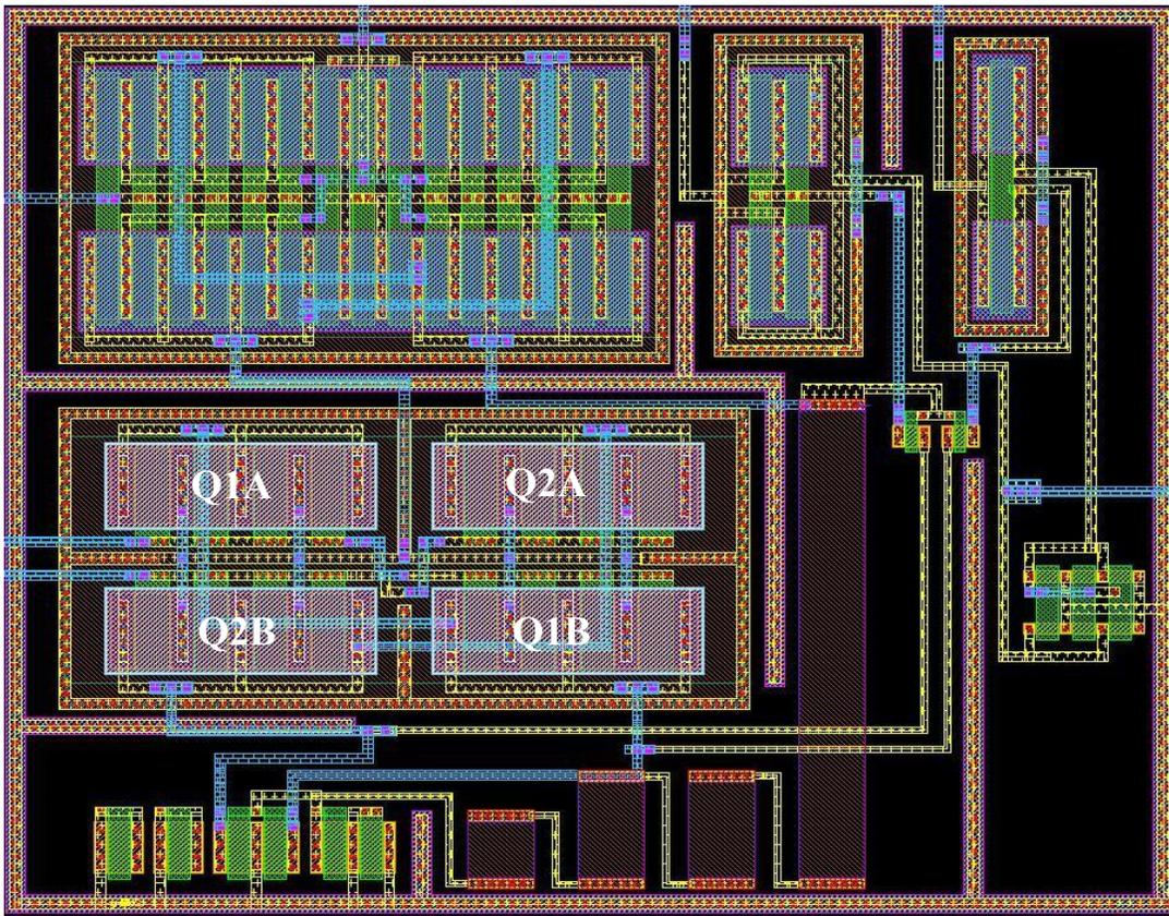
Figure 2.18 Layout of the voltage comparator
