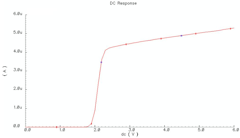
Figure 2.7 Current source power supply dependence (typ.)
