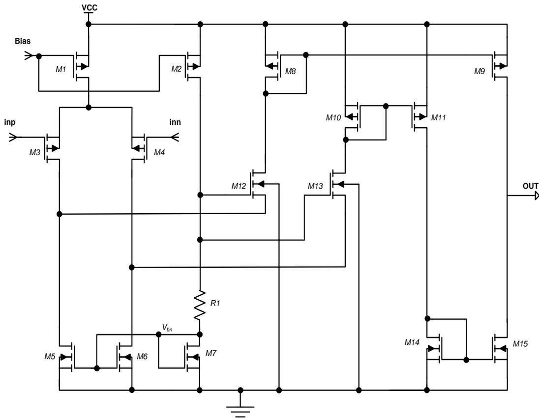
Figure 2.12 Schematic of the voltage comparator
