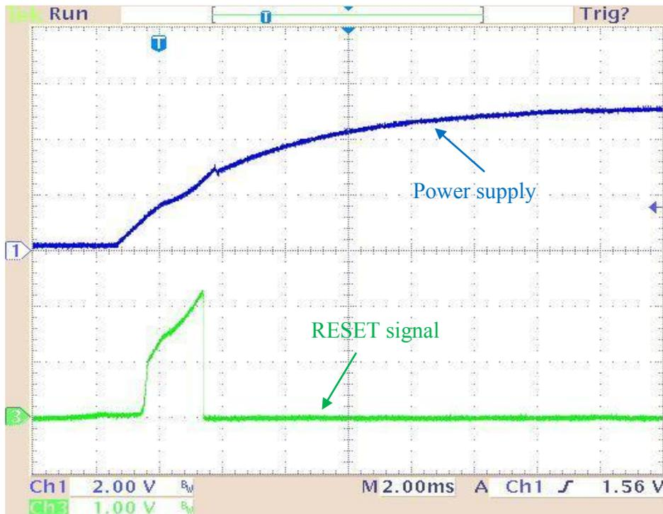
Figure 2.21 UVLO at Power-up transient
