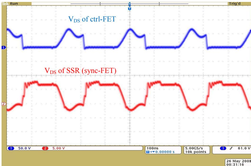
Figure 3.8 Operating waveforms at 4MHz
