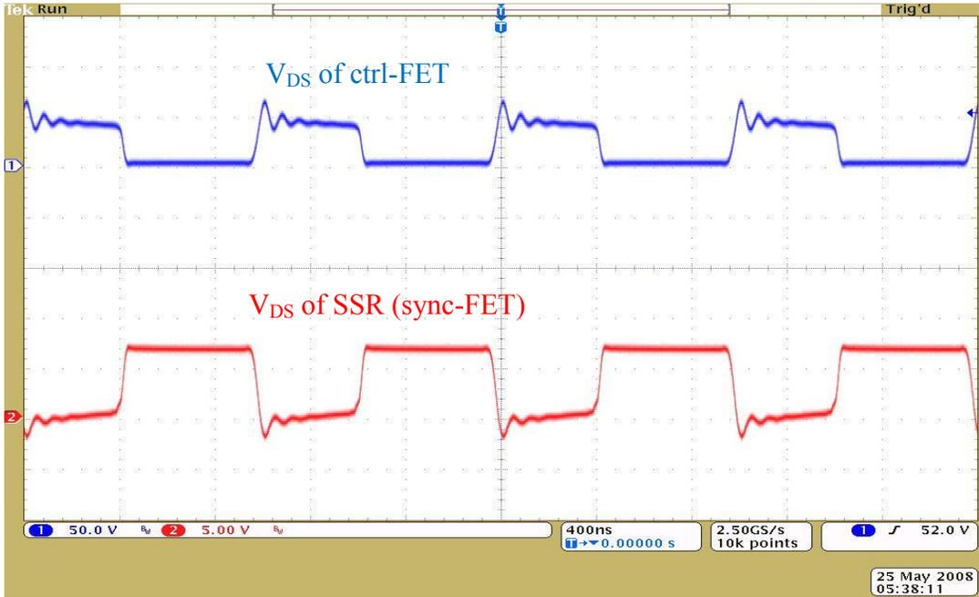
Figure 3.6 Operating waveforms at 1MHz
