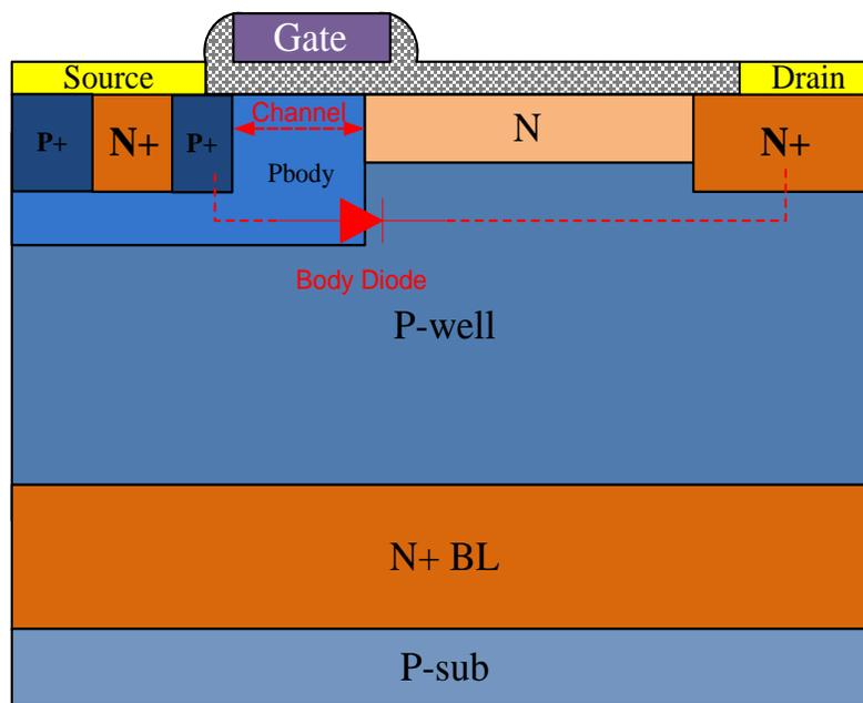
Figure 1.1 A typical power MOSFET structure with the inherent body diode
