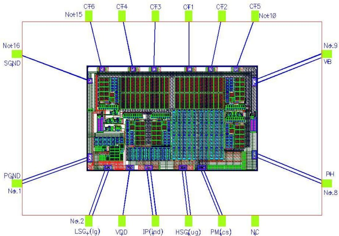
Figure 4.11 CSD chip bonding diagram
