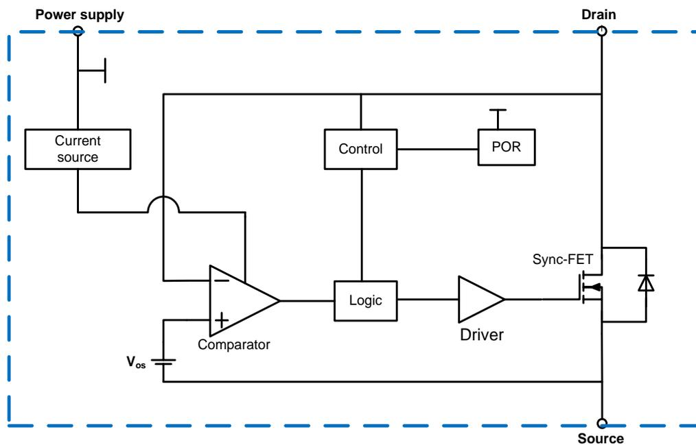
Figure 2.3 Block diagram of the proposed self-synchronous rectifier
