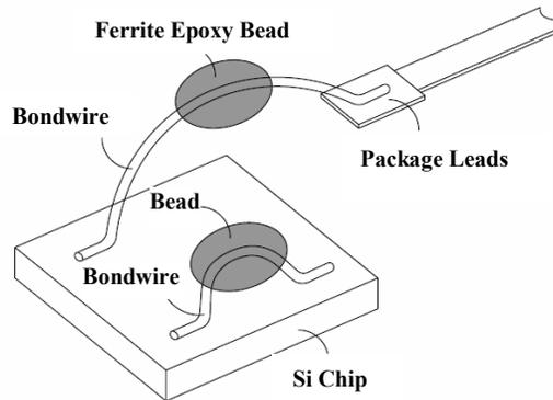
Figure 5.1 Concept of single bondwire with ferrite epoxy beads
