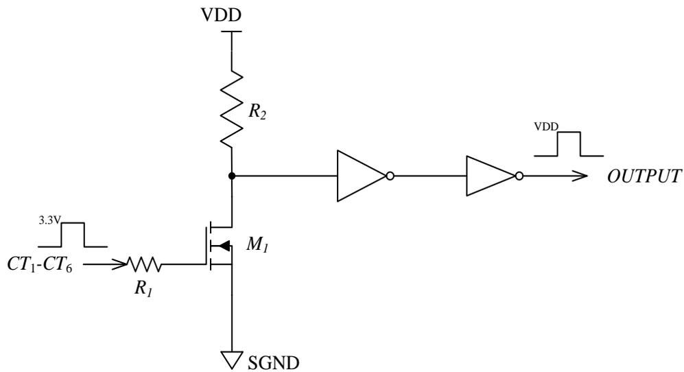
Figure 4.6 1<sup>st</sup> Level shifter
