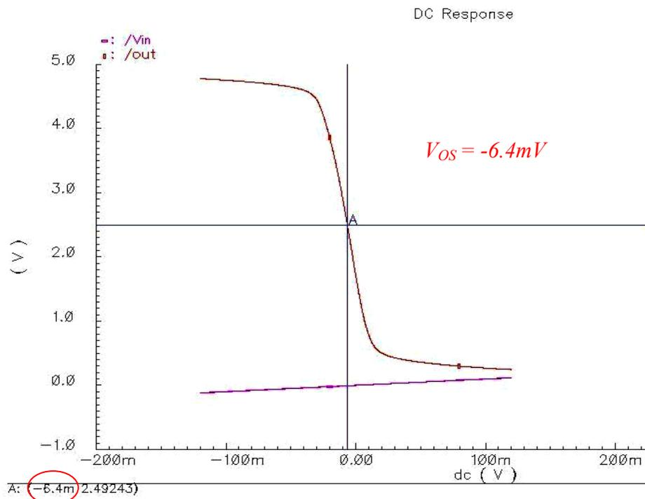
Figure 2.14 Voltage comparator offset voltage simulation
