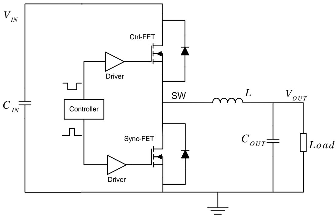
Figure 2.1 Conventional synchronous buck converter
