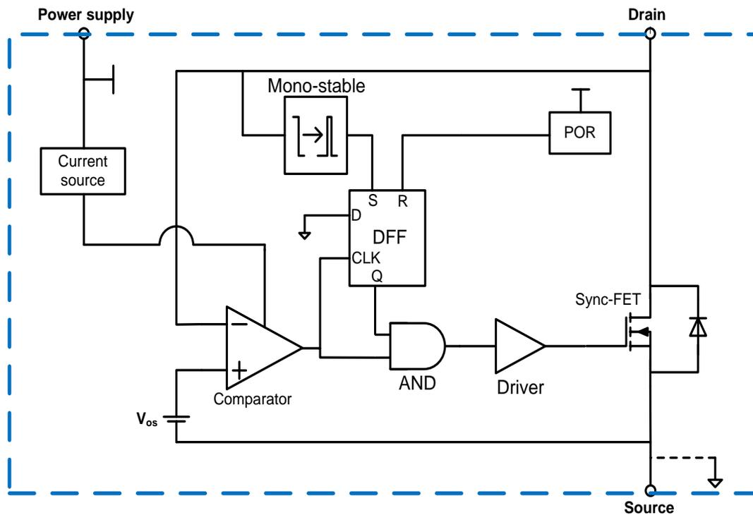
Figure 2.15 Detailed block diagram of the proposed SSR with the ONE-SHOT control
