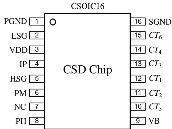
Figure 4.12 CSD chip pinouts
