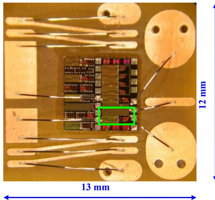
Figure 5.5 The buck PSiP before ferrite epoxy coating
