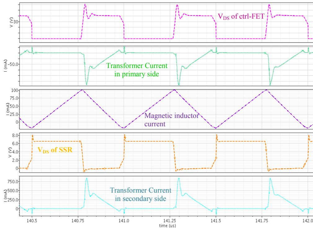
Figure 3.4 DCM Simulation results
