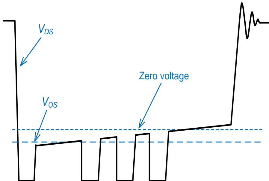
Figure 2.11  $V_{DS}$  waveform with oscillation for  $V_{OS} < 0$  under light load
