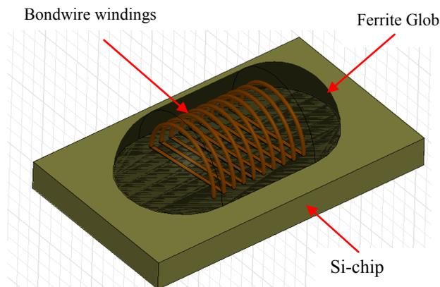
Figure 5.2 Concept of coupled on-chip multi-turn bondwire inductor
