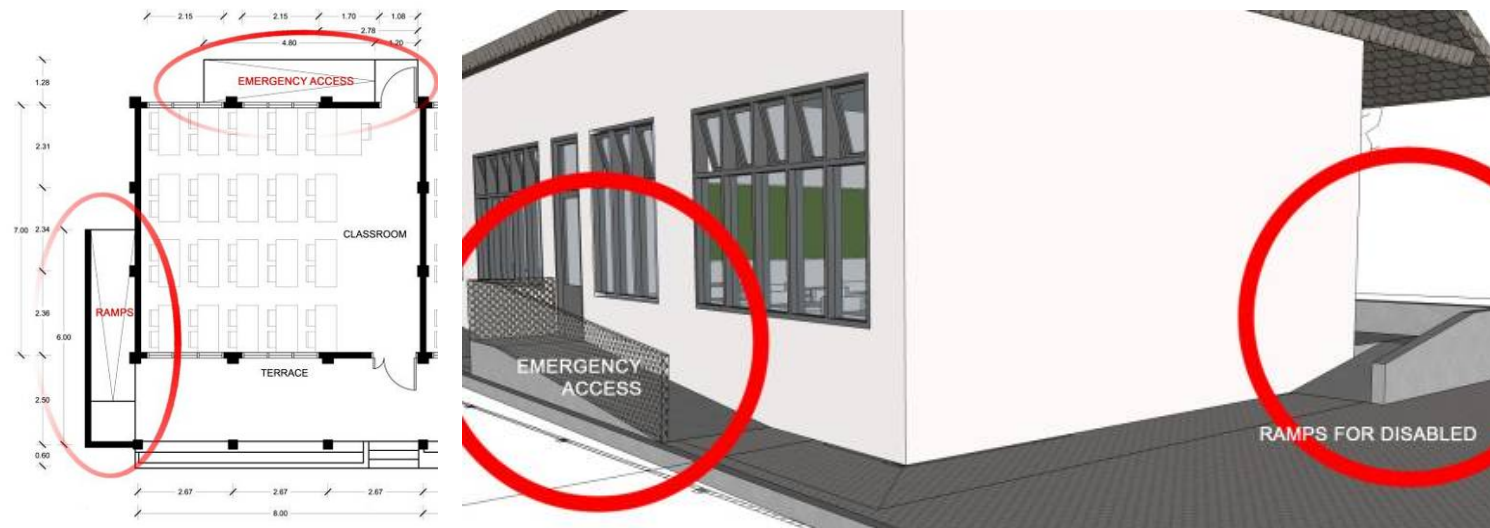
Figure 16 Ramps and Emergency Access From Classroom (left) and Ramps and Emergency Exit Area (right)
