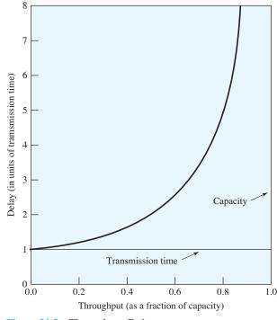
Figure 21.5 Throughput Delay
