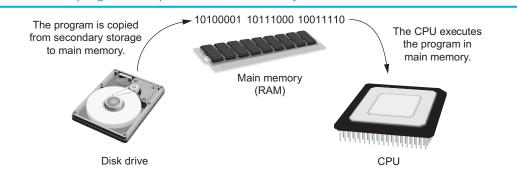
When a CPU executes the instructions in a program, it is engaged in a process that is known as the *fetch-decode-execute cycle*. This cycle, which consists of three steps, is repeated for each instruction in the program. The steps are:
