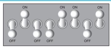
When a piece of data is stored in a byte, the computer sets the eight bits to an on/off pattern that represents the data. For example, the pattern shown on the left in Figure 1-8 shows how the number 77 would be stored in a byte, and the pattern on the right shows how the letter A would be stored in a byte. We explain below how these patterns are determined.
