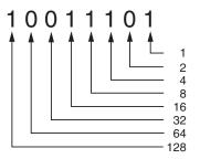
To determine the value of a binary number you simply add up the position values of all the 1s. For example, in the binary number 10011101, the position values of the 1s are 1, 4, 8, 16, and 128. This is shown in Figure 1-11. The sum of all of these position values is 157. So, the value of the binary number 10011101 is 157.
