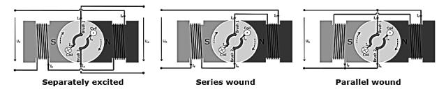
Figure 31: Overview of the three different DC-motor types
