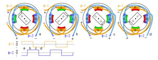
Figure 67: Simplified permanent magnet stepper in full-step drive (31)
