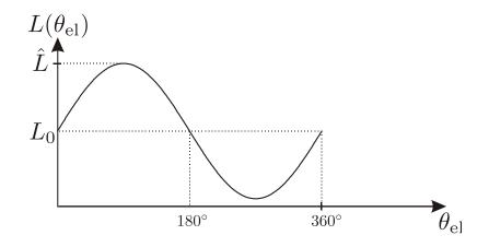
Figure 89: VR-Resolver: Change of inductance as function of the rotor position (5)
