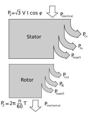
Figure 96: Breakdown example of losses in an electric machine, e.g. induction machine (5) (53)
