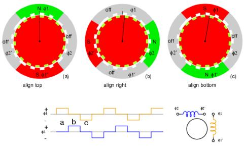
Figure 71: Hybrid stepper motor rotation sequence (31)
