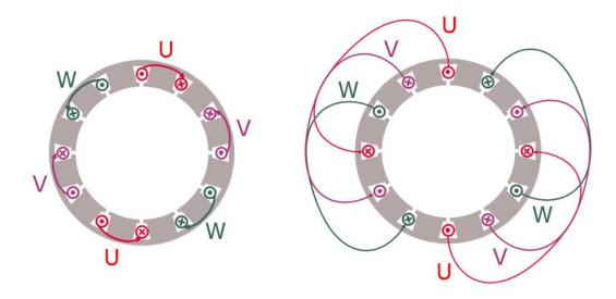
Figure 21: Concentrated (left) vs. distributed (right) winding system
