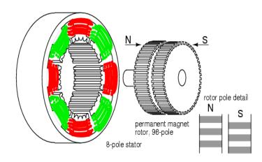
Figure 69: Hybrid synchronous stepper motor (31)
