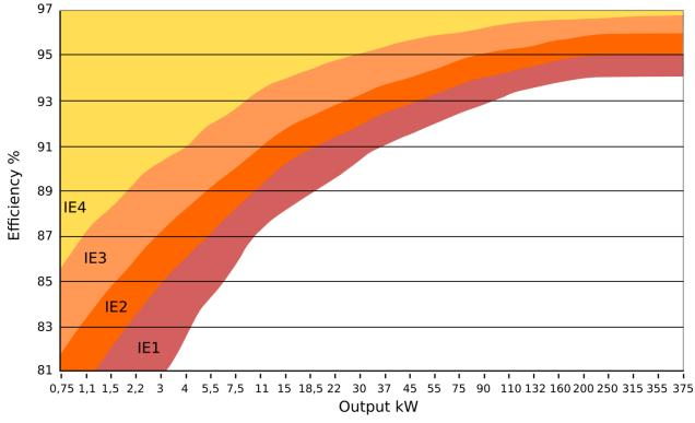
Figure 98: IE efficiency classes for 4-pole (2 pole pairs) motors at 50 Hz (5) (57)
