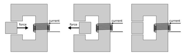
Figure 80: Reluctance force in a magnetic circuit (5)
