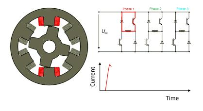
Figure 52: Current flow of the free-wheeling state (5)
