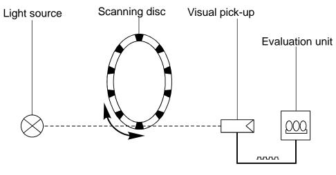
Figure 84: Optical incremental position encoder (5)
