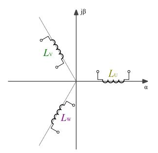
Figure 90: Arrangement of the  $\alpha\beta$ -coordinate system (48)
