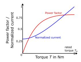
Figure 14: Normalized current and power factor over torque (5)
