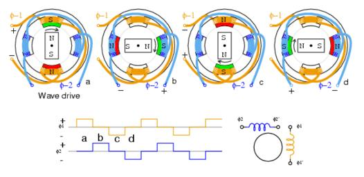
Figure 66: Simplified permanent magnet stepper in wave drive (31)
