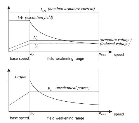
Figure 37: Operating limits of the separately excited DC machine (5)
