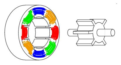
Figure 61: Variable reluctance stepper motor (31)
