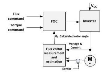
Figure 94: Block diagram of direct field-oriented control (DFOC) (50)
