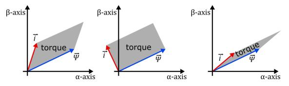
Figure 79: Relationship between current / flux linkage space vectors and torque (5)
