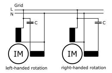
Figure 18: One-phase induction motor as capacitor motor (5)
