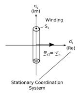
Figure 81: Producing flux linkage with one winding (5)
