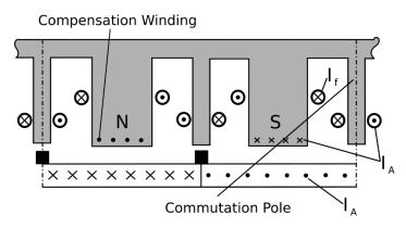
Figure 30: Compensation windings and commutation pole of a separately excited DC machine (5)
