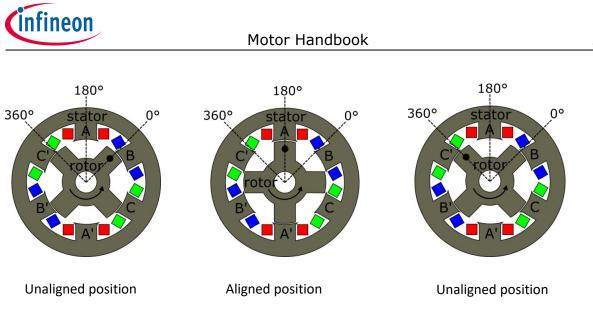
Figure 54: Electrical cycle for phase "A" (7; 5)
