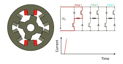
Figure 51: Current flow of the magnetization state (5)
