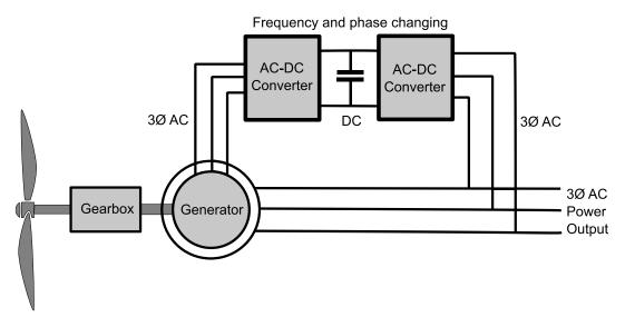
Figure 17: Doubly-fed induction generator connected to a wind turbine (11)
