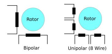
Figure 72: Bipolar and unipolar winding arrangements (34)
