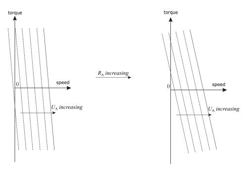
Figure 33: Torque-speed characteristic curves of a separately excited DC machine (5)
