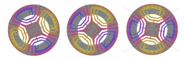
Figure 25: Magnetic flux paths within the synchronous reluctance machine with anticlockwise rotation (5)
