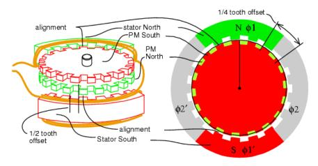
Figure 70: Simplification of hybrid stepper motor (31)
