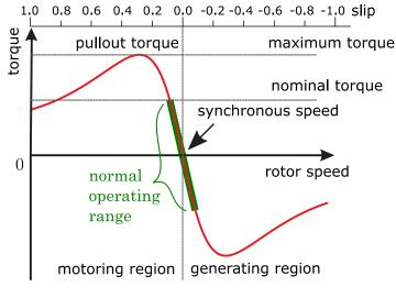
Figure 6: Torque-vs.-speed diagram of the IM (5)
