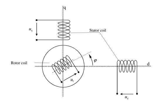
Figure 87: Resolver for absolute position measurement (5)
