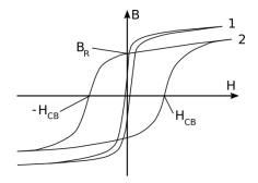
Figure 97: B(H)-characteristic of magnetic materials (5) (55) 1 = soft-magnetic material, e.g. iron 2 = hard-magnetic material, e.g. permanent magnets
