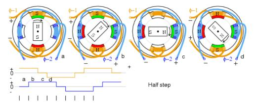
Figure 68: Simplified permanent stepper motor in half step drive (31)
