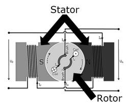
Figure 29: Schematic representation of an electrically excited DC machine (here: "separately excited")
