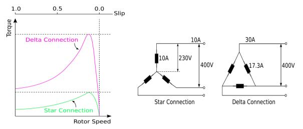
Figure 9: Star- and delta-connected IM (5)
