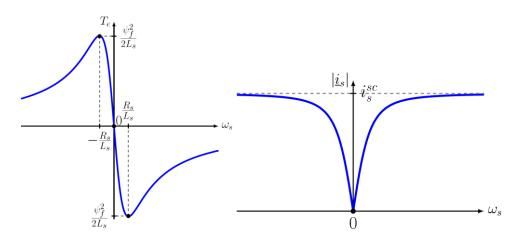
Figure 23: Short circuit torque and current compared to rotor speed (5) (7)
