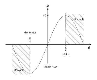
Figure 22: Torque as a function of load angle at constant voltage operation (5)
