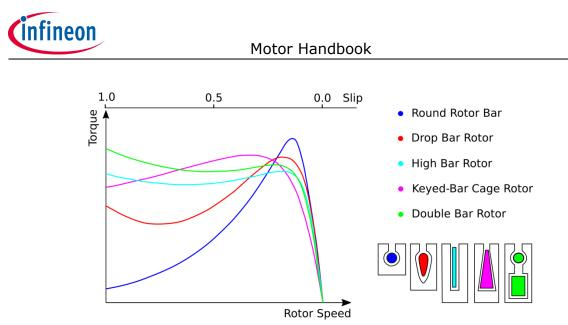
Figure 8: Influence of the shape of rotor bars (5), (6)
