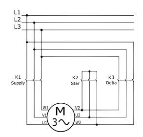
Figure 10: Star-Delta-Switching using contactors (5)
