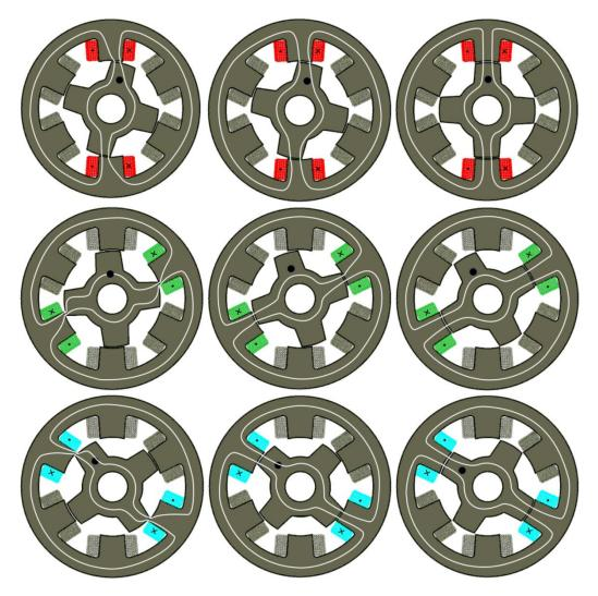
Figure 47: Continuous rotation of switched reluctance motors (5)
