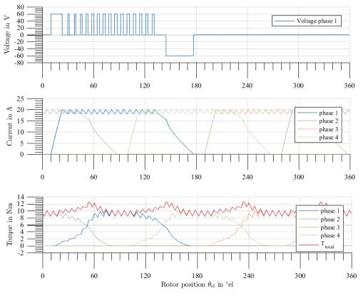
Figure 55: Operating in low speed (7; 5)
