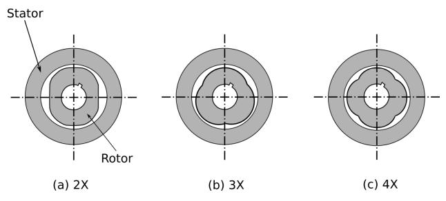
Figure 88: Examples of rotor shapes of the VR-type resolvers (5)
