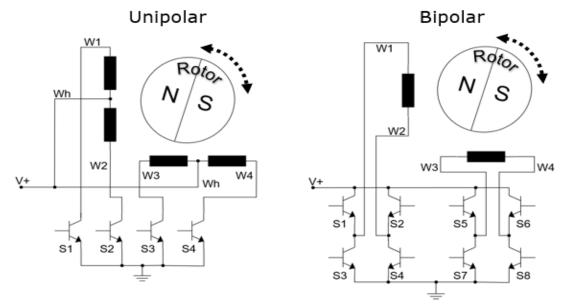
Figure 73: Switches for bipolar and unipolar motor (36)
