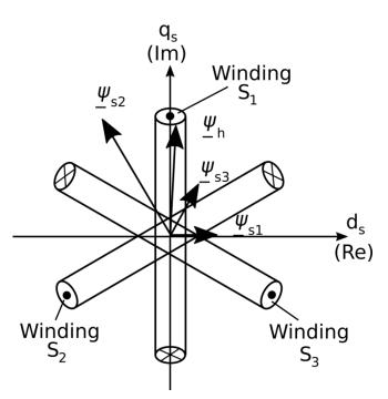
Figure 82: Flux linkage of a three-phase system (5)
