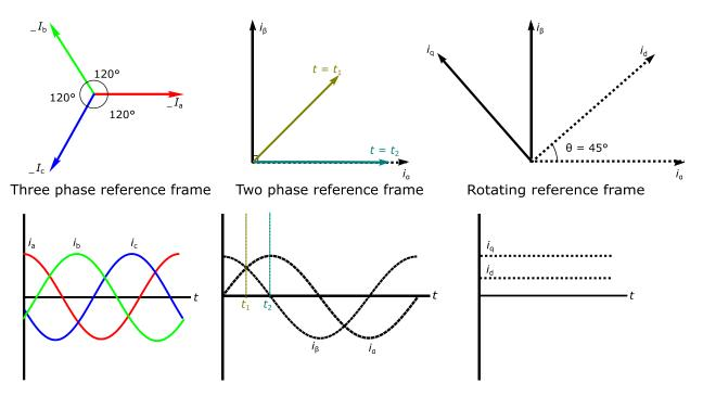
Figure 91: Transformations of a three-phase system (5)
