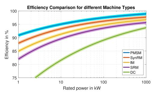
Figure 100: Example comparison of efficiency for different machines (60), (61)
