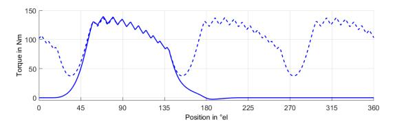
Figure 57: Torque production of a three-phase SRM (5)
