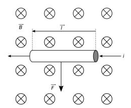
Figure 77: Lorentz force on a current carrying conductor in a magnetic field (5)
