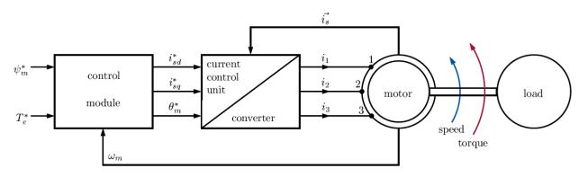
Figure 92: Field-oriented control drive structure (7)
