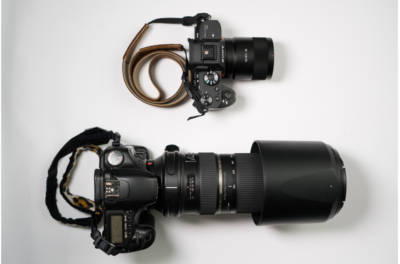
Mirrorless camera (top) versus a DSLR (bottom) as a size comparison.
