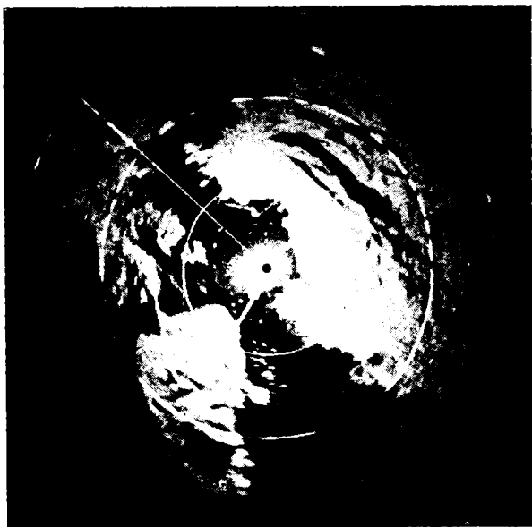
FIG. 7-2.—Radar plan-position indicator with range and azimuth markers.
