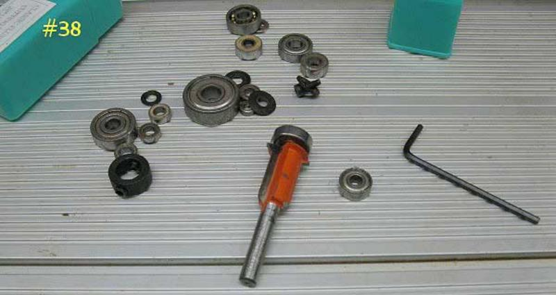
the original bearing, on the right would have made for too deep a groove, so replaced with a bigger one as shown
