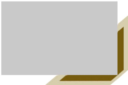
Note that on the short edge, the board is one board's thickness away from the edge of the leather, and that the leather has been pared back one boards thickness.
