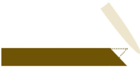
The 45 degree cut has to be pressed down onto the board, use your bone folder.
