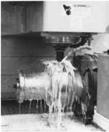
(b) Milling cylindrical cam.
