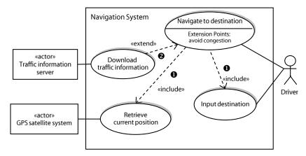
Figure 6-4 An example using modeling elements of use case diagrams
