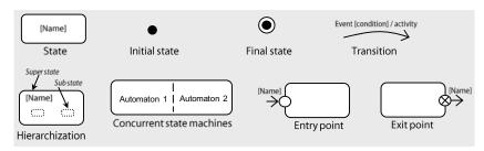
Figure 6-17 Modeling elements of state machines as defined by the UML 2
