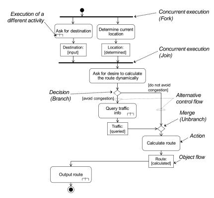
Figure 6-13 Activity diagram in UML notation
