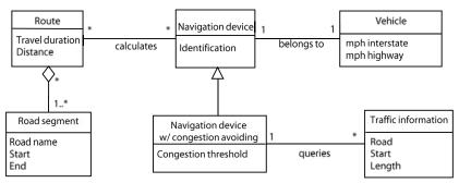
Figure 6-9 Class diagram in UML notation
