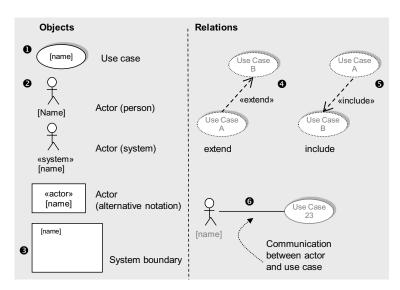
Figure 6-3 Essential modeling elements of use case diagrams
