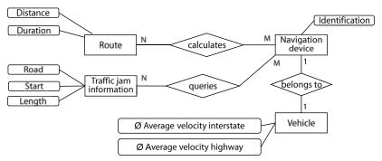
**Figure 6-7** Entity-relationship diagram (data model) according to Chen
