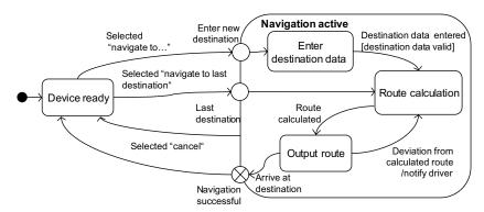
Figure 6-18 State diagram in UML 2 notation
