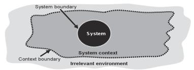
Figure 2-1 System and context boundary of a system
