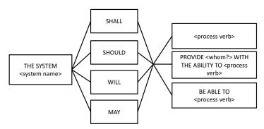
Figure 5-2 The core of a requirement and its legal obligation
