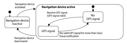
Figure 6-16 Simplified statechart of a vehicular navigation device
