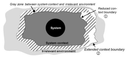
Figure 2-4 Gray zone between system context and irrelevant environment
