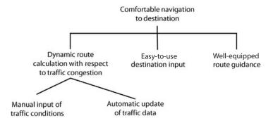
**Figure 6-2** Goal model in the form of an AND/OR tree
