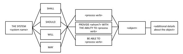
Figure 5-3 Principle of a complete requirements template without conditions
