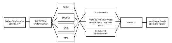
Figure 5-4 The complete requirements template with conditions
