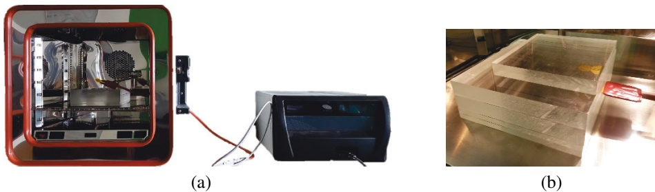
Figure 3.4 TPS experimental setup: (a) Setup with climate chamber. (b) Measurement of PMMA.
