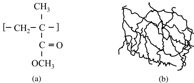
Figure 2.7 (a) repeating unit of MMA ( \text{CH}_2 = \text{C}(\text{CH}_3)\text{COOCH}_3 ); (b) molecular structure of PMMA.
