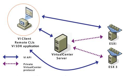
Figure 4: Using the VMware Virtual Infrastructure API in a VMware Infrastructure environment
