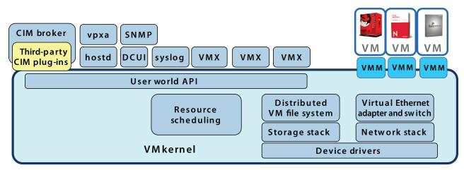
Figure 1: The streamlined architecture of VMware ESXi eliminates the need for a service console.
