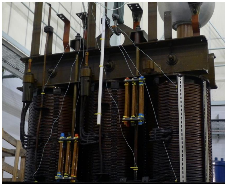
Figure 4-18 Front view of the active portion of the transformer, after installation of thermocouples, moisture sensor and pre-conditioned paper samples
