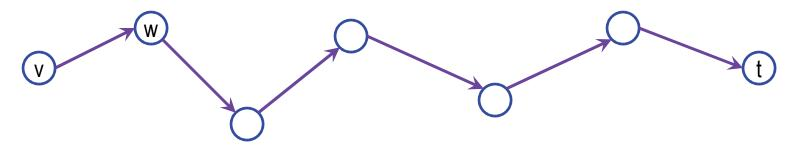
Shortest v - t path can use i - 1 arcs. Then OPT(i,v) = OPT(i - 1,v)Or it can use i arcs and the first arc is vw. Then OPT(i,v) = len(vw) + OPT(i - 1,w)
