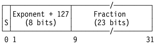
Figure 19-4. BFP Short Format (4 bytes)
